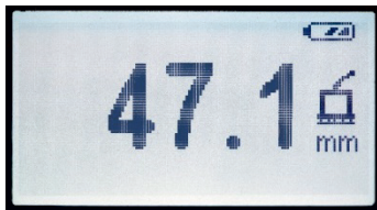
Image 13: Current measured value with coupling symbol
