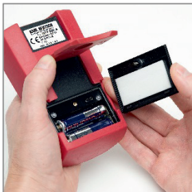
Image 6: Opening the battery compartment
