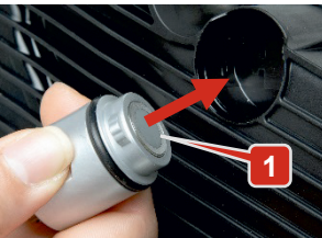
Image 9: Probe before insertion into the transmission oil sump socket
