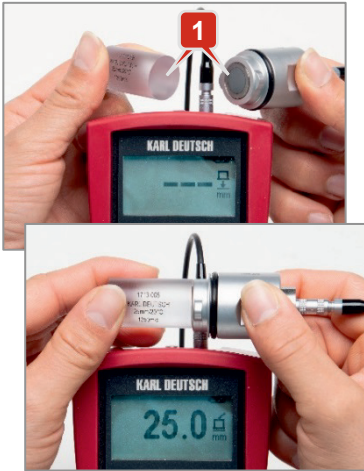
Image 15: Measurement on the test block as regular control measurement
