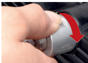
Image 11: To lock the probe, push it in and turn it to the right
