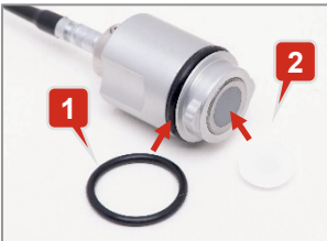
Image 8: View of the probe with O-ring (1) and round protective disc (2)
