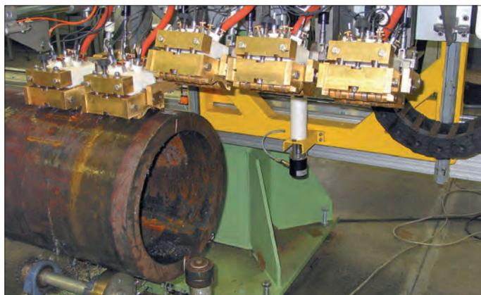
Inspection of tubes with 5 incidence directions: In this example, 5 ultrasonic probes are mounted into each probe holder, which individually may be lowered and lifted for short untested tube ends. Water jet coupling is employed to obtain stable coupling conditions. Longitudinal and transverse defects are detected with angular incidence. The testing angle is typically chosen to 45° within the tube material. Straight beam testing is used to detect laminations and to measure the wall thickness.
