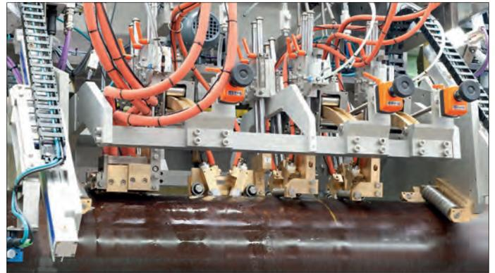
In this example ten probes are used for offline weld testing. The six angle beam probes use water jet coupling (also called squirter technique). The incidence angle can be adjusted without steps for a perfect setting with respect to pipe diameter and wall thickness and without changing the probe.
