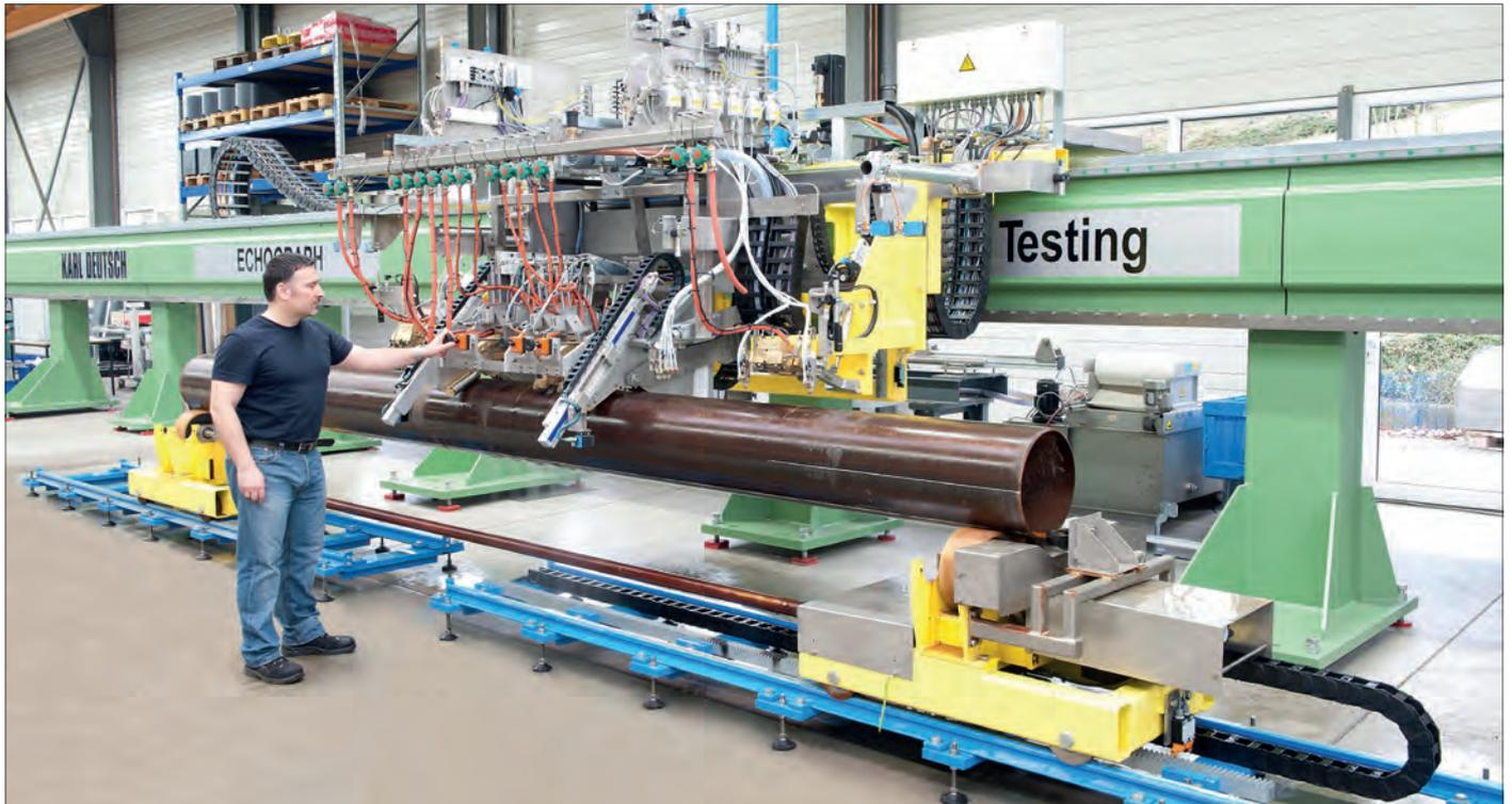
Test portal (offline test machine) during assembly at the KARL DEUTSCH workshop
