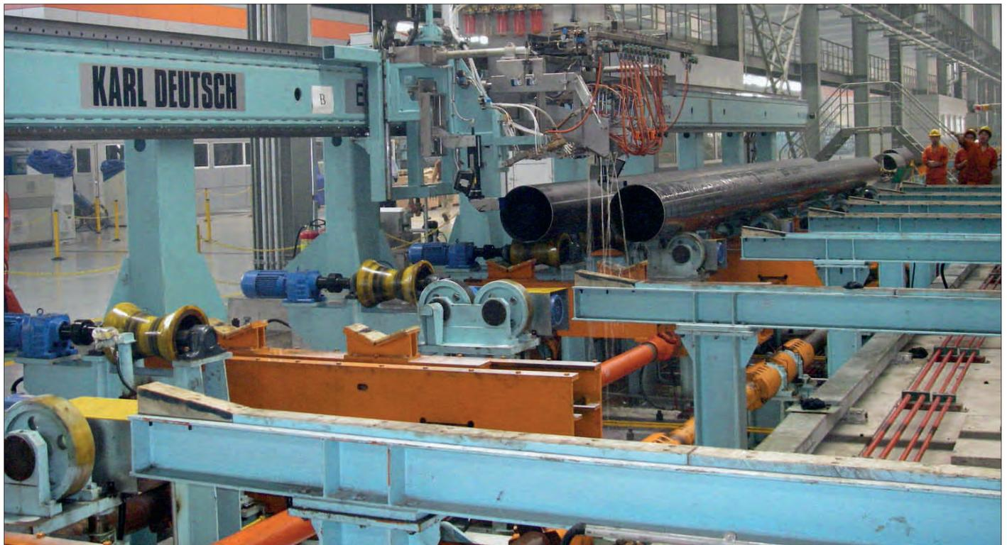
Test portal (offline test machine): Onsite operation with transverse conveyor for pipe feeding and linear discharging of the pipes. This machine was also equipped with two additional probe holders for the pipe end inspection.
