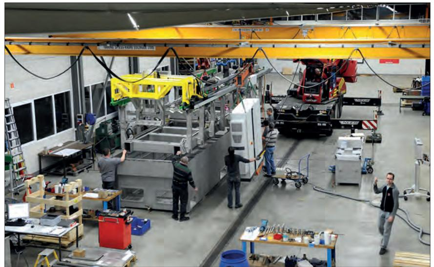
View into the systems workshop where a large immersion test tank is being assembled
