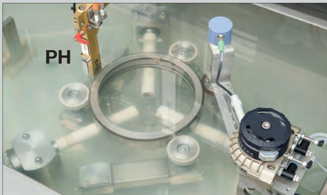
View into immersion tank with bearing ring: The probe holder (PH) is positioned outside the ring to inspect the internal ring surface. For higher throughput, four probes are used in parallel for the inspection. The ring is put into rotation with three rollers. A vertical probe movement results in helical test tracks.
