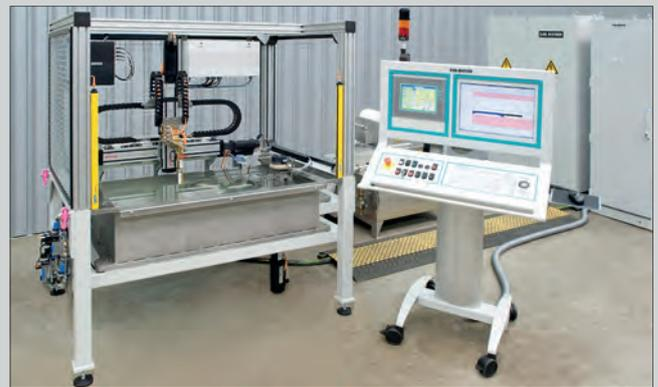
ECHOGRAPH test electronics with immersion tank, probe manipulator and water filter circulation system: The operator panel contains a touch screen for setting the PLC parameters and an industrial keyboard to set the ultrasonics.
