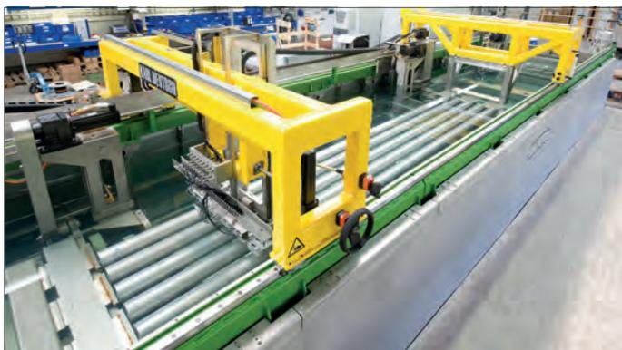
Large immersion test tank for bars, profiles and tubes. Up to six samples can be tested at the same time.
