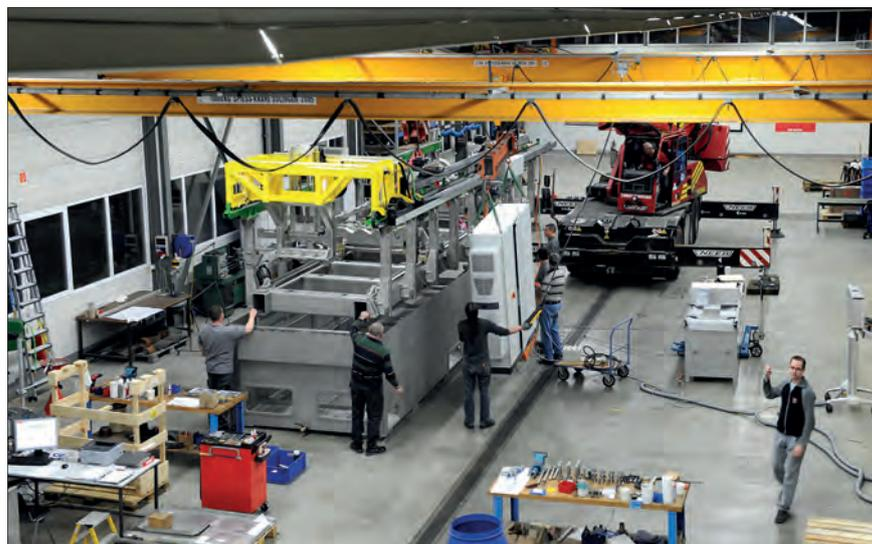
View into the systems workshop where a large immersion test tank is being assembled
