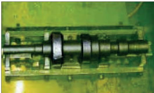
Testing of forged gear shafts (chevrons)
