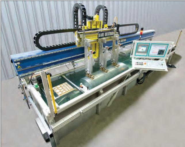
Test tank for rotational aluminium billet inspection
