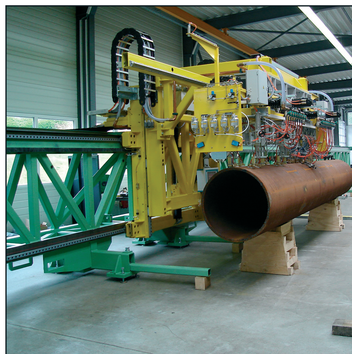
Moving Probes (1 m/s) and Resting Pipe
