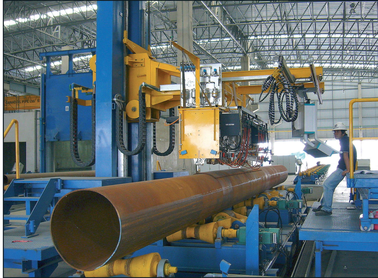
Weld Testing with Stationary Machine Stand and Moving Pipe
