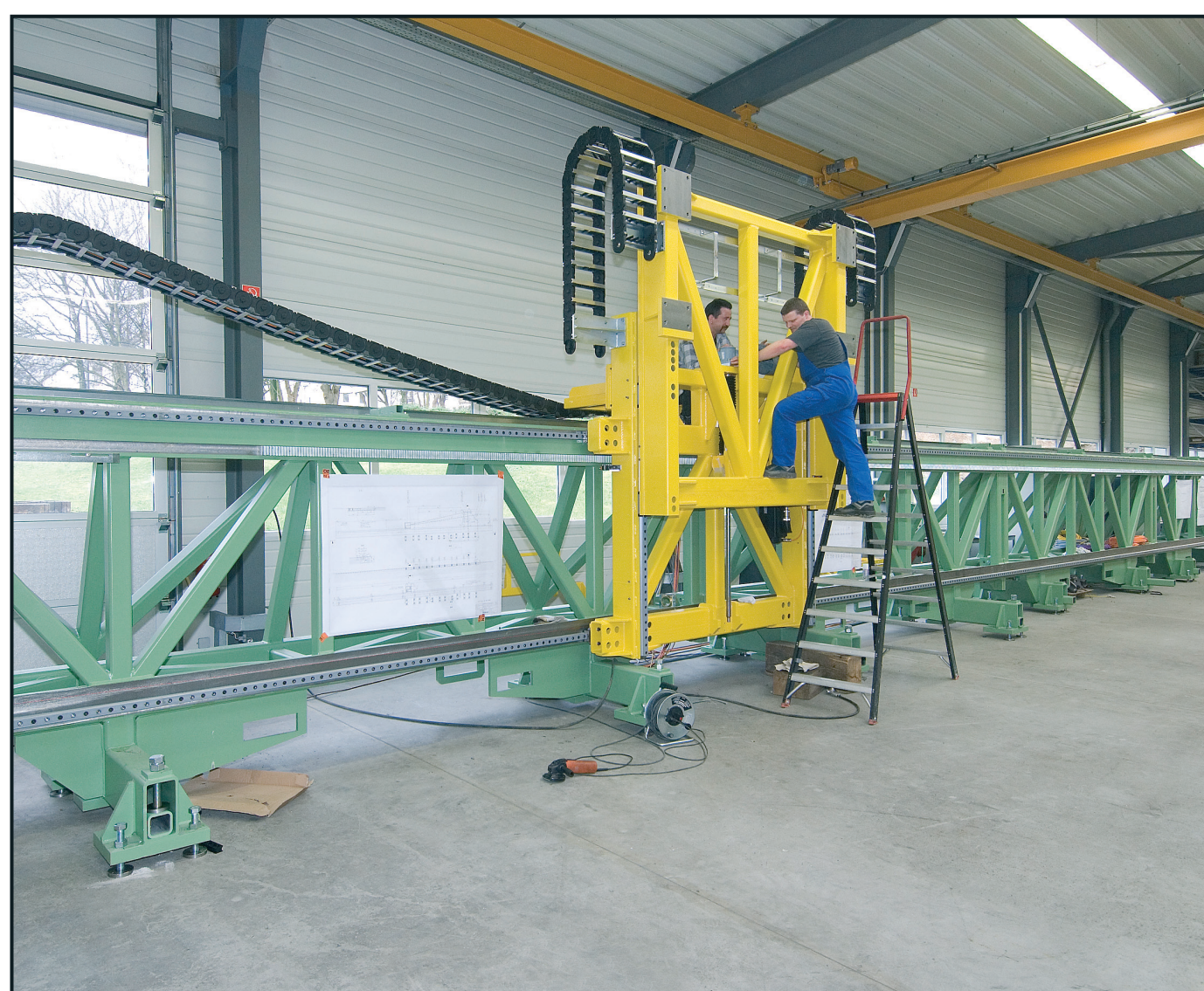
Test Portal Assembly at KARL DEUTSCH Systems Workshop
