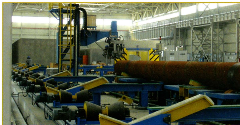
Figure 7. Weld testing system with machine stand and pipe before testing.
