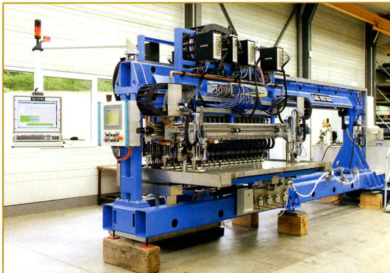
Figure 4. Strip testing machine with calibration unit. In this image, all probes are moved above a test plate. The plate support is motorized to perform a dynamic check of the calibration.
