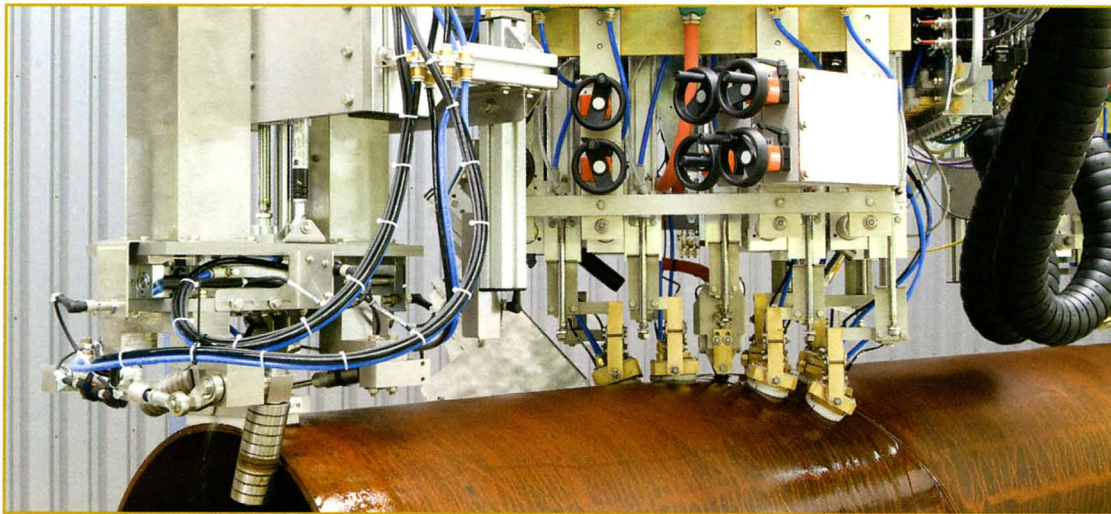
Figure 8. Final ultrasonic test of weld with 10 probes and both pipe ends with two-channel probe.
