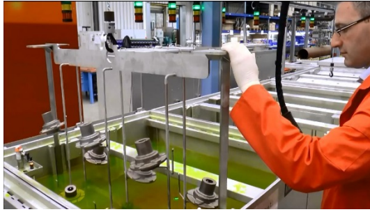
Fig. 9. Placement of the workpiece holder into the penetrant tank (due to a non-disclosure agreement the original components cannot be shown)
