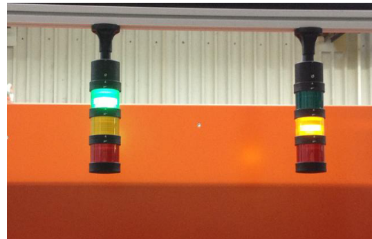
Fig. 14. Signal lamps show the status of each station (green: station waiting, yellow: station working, yellow blinking: station ready)
