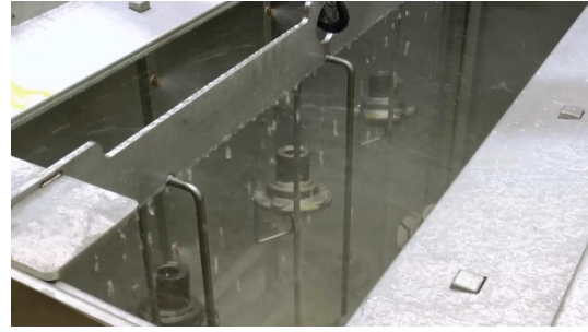
Fig. 10. Penetrant removal with water jets
