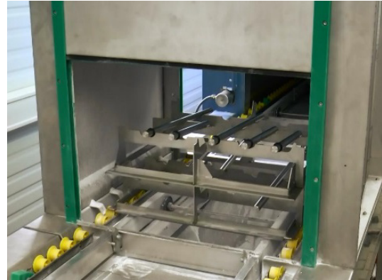
Fig. 6. Dry developer application in a vortex chamber
