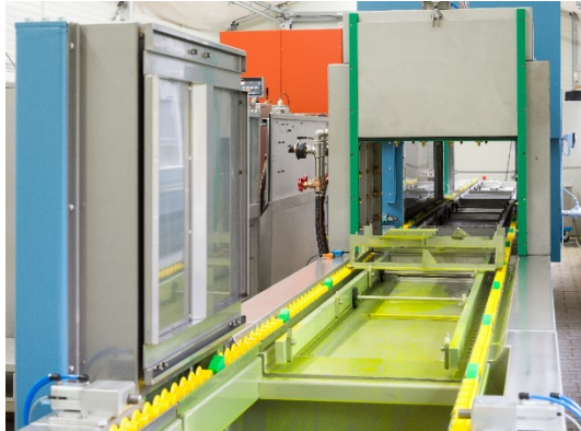
Fig. 5. Workpiece holder just before passing into the water jet tunnel for penetrant removal
