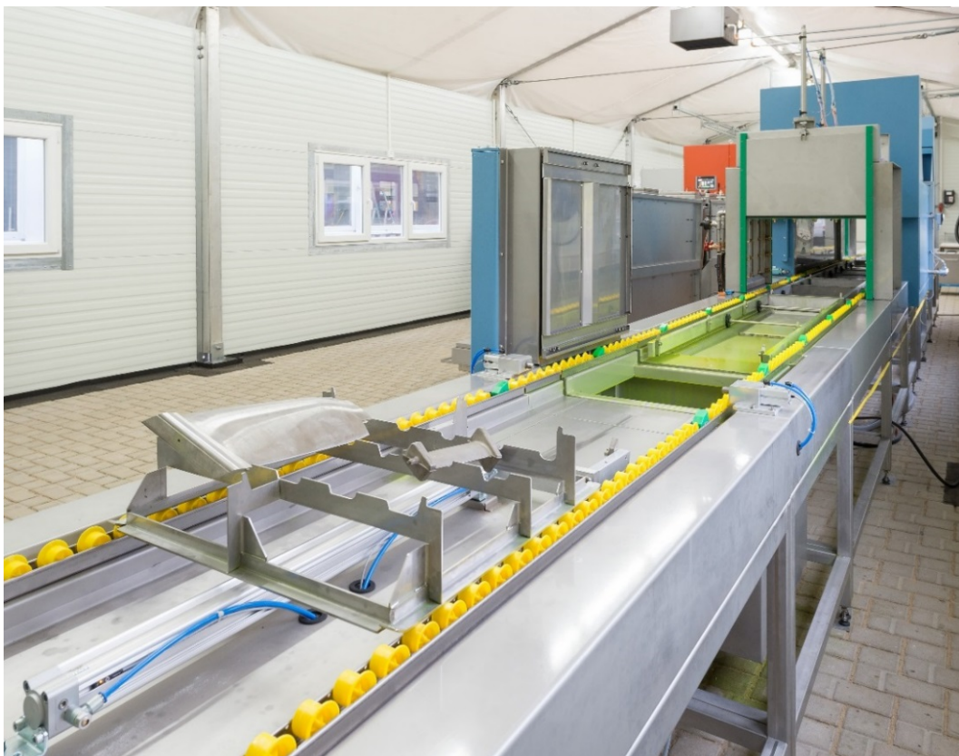
Fig. 4. Fully automated testing system for forgings (due to a non-disclosure agreement the original components cannot be shown)
