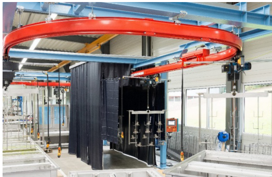
Fig. 13. Cabin for visual evaluation. The workpiece holder with a capacity of up to 24 parts is hanging at one of the nine crabs.
