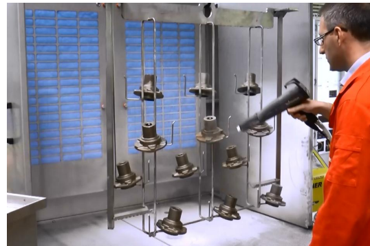
Fig. 12. Electrostatic dry developer application
