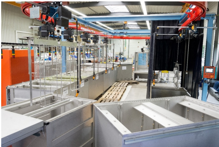
Fig. 8. Semi-automated testing system with oval crane runway
