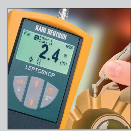
Coating Thickness Measurement
