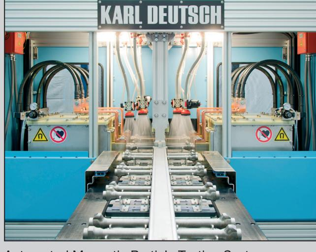
Automated Magnetic Particle Testing System
