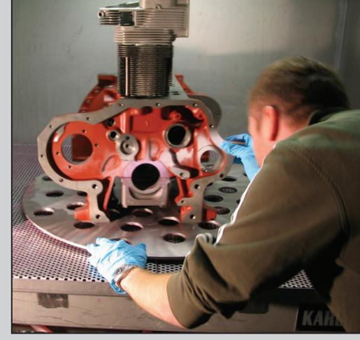
Penetrant Testing of Motor Block
