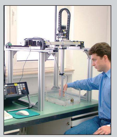
Final Test of Ultrasonic Probes
