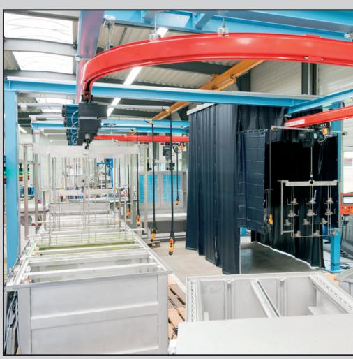
Large Dye Penetrant Testing System
