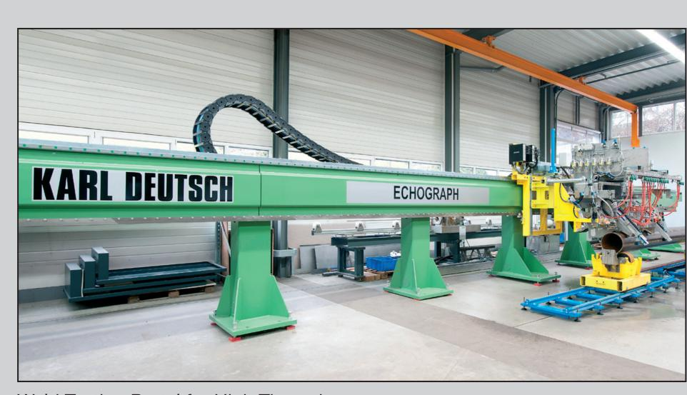
Weld Testing Portal for High Throughput
