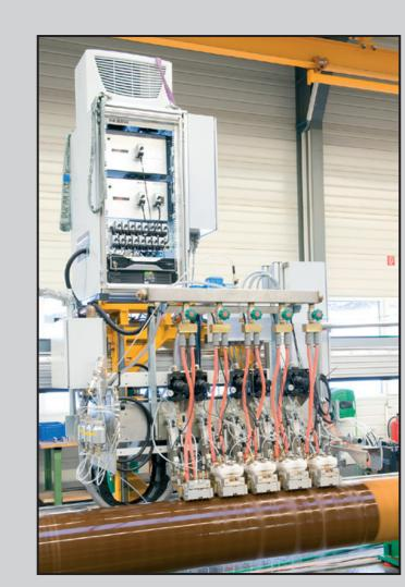
Phased Array Tube Testing
