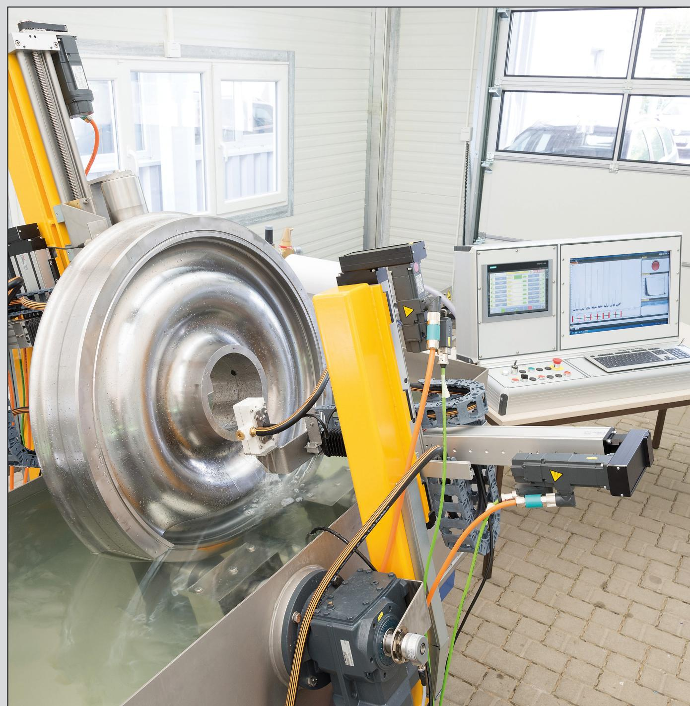
Wheel Testing within one Rotation with 384 Parallel Phased Array Channels
