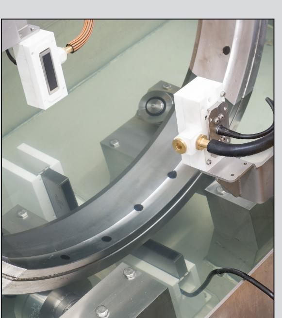
Immersion Testing of Tread and Rim (2 Arrays)
