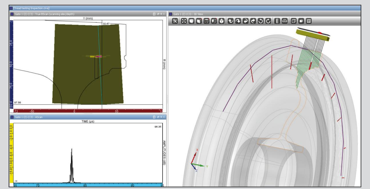
CIVA Simulation for Tread Testing: B-Scan & A-Scan of Flat-Bottom Hole, 3D-View of Test Wheel
