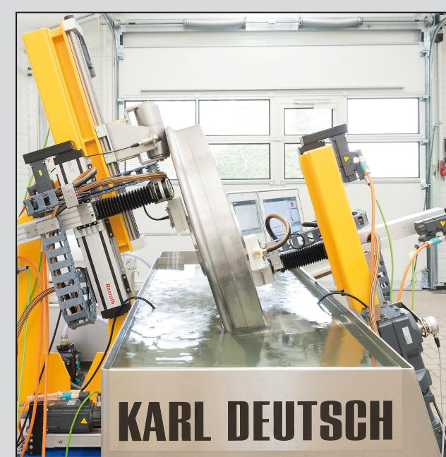
Two-Sided Hub Testing (2 Arrays)
