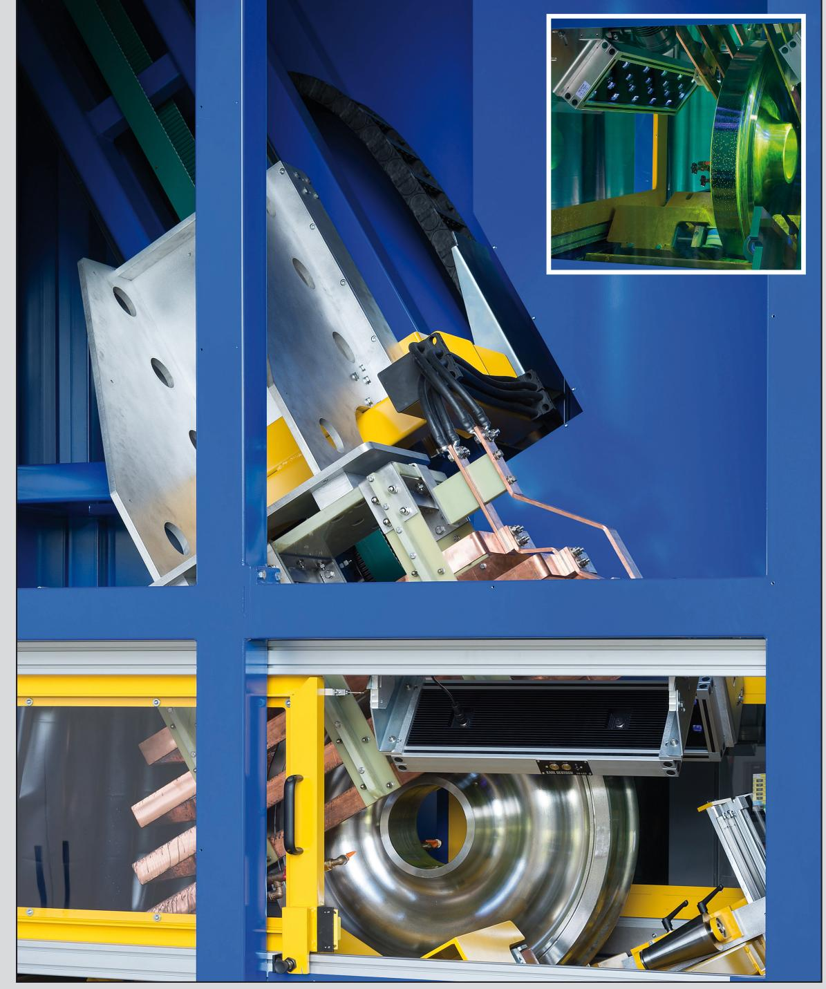
Total View with Loading Position (Left), Magnetization Unit and Darkroom Cabin
