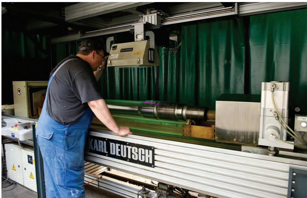
**Figure Visual Test.** Motorized roller unit for convenient viewing of the axle under UV-light. The UV-lamp can easily be moved into the correct axial position.
