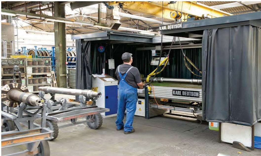
**Figure Loading and Unloading.** The roof of the test cabin can be pneumatically opened and closed. The UV-lamp is then moved backwards into the safety position.
