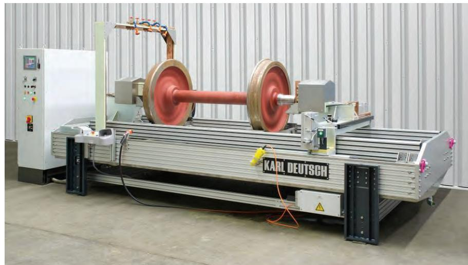
**Figure Wheelset Test.** Inspection of the axles where the wheels are still mounted (at S.C. Remar S.A in Iasi). Of course, a test for surface cracks can not be carried out in lacquered condition as seen on photograph.
