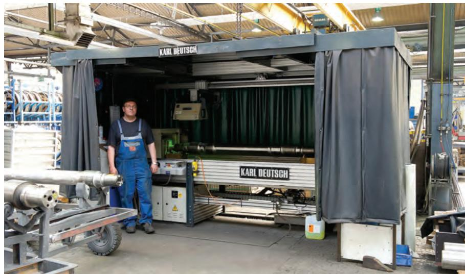
**Figure Axe Testing System.** Magnetic particle testing of railway axles at Deutsche Bahn in Krefeld, Germany.
