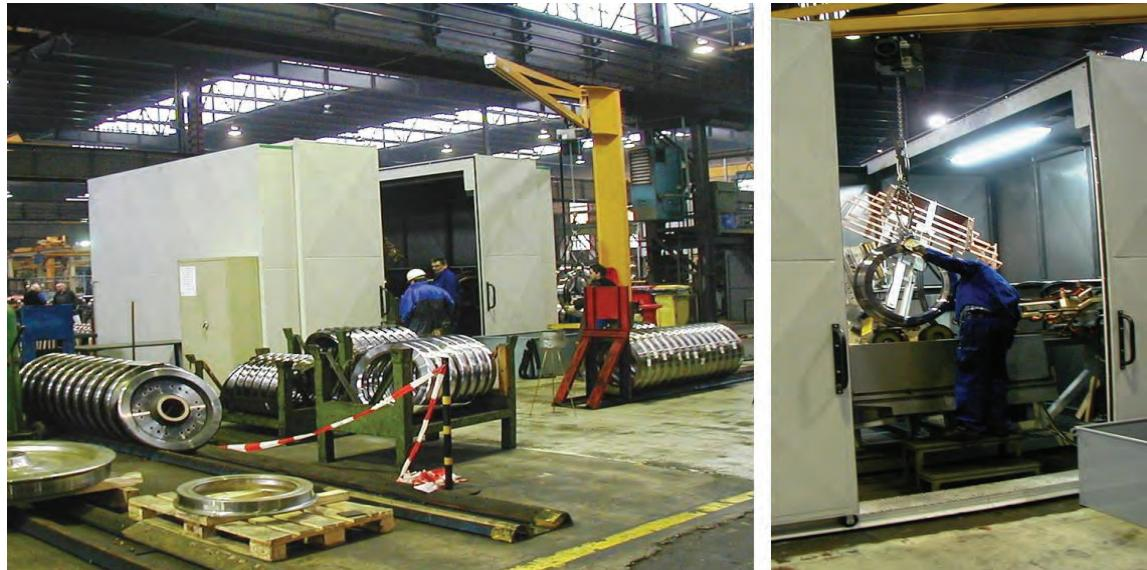
**Figure MT-Wheel Testing System.** Loading of wheel rims by means of a crane at the company Bochumer Verein Verkehrstechnik GmbH.
