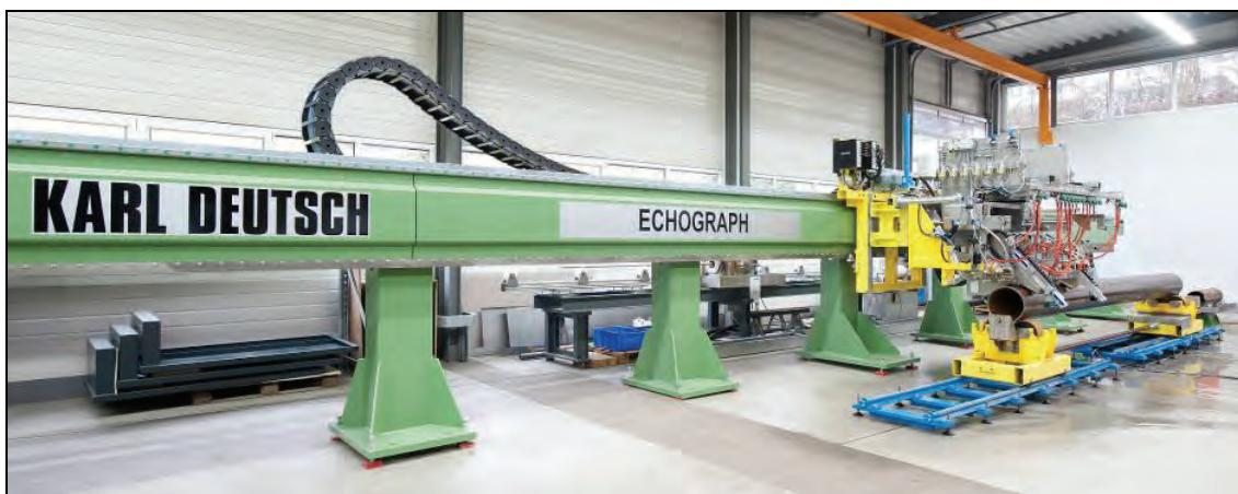
**Figure Final Pipe Weld Test.** Offline weld testing portal (type ECHOGRAPH-SNHFT).
