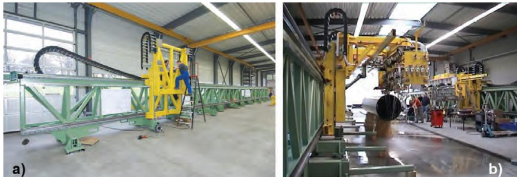
**Final Assembly of two weld testing systems,** a) Assembly of two systems with a total length of 35 m, b) Check of the testing system with a sample tube at full testing speed.
