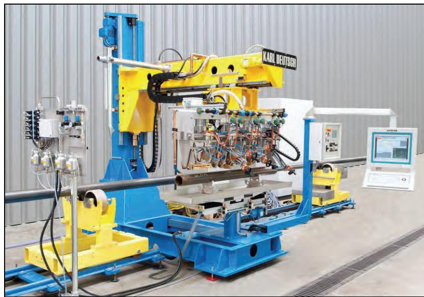
**Figure Test Mechanics (Online Test).** Stationary machine frame with probe holders in the calibration position.
