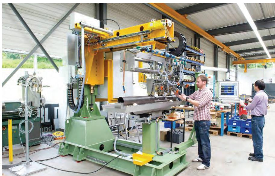
**Figure Phased Array Testing Machine.** System before shipment in KARL DEUTSCH workshop.
