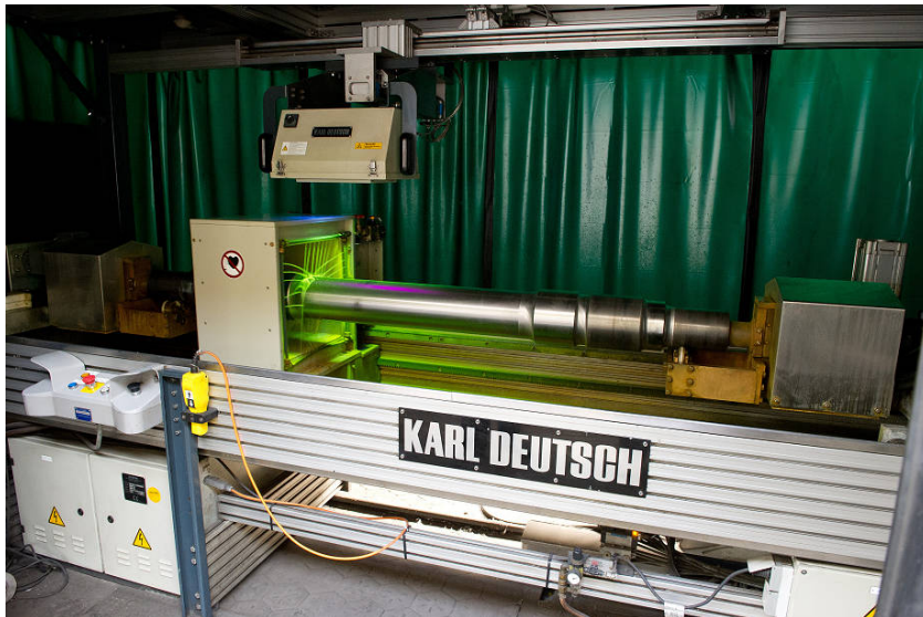
Figure 4. Magnetization of a railway axle shaft with a motorised moving coil
