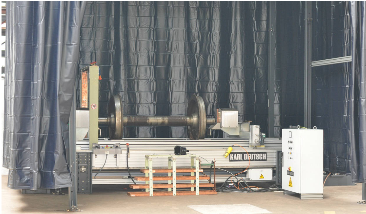
Figure 11. DEUTROFLUX UWS for testing railway axle while the wheels are still mounted In front of the test machine is the separate test coil “Mindener Coil” for testing the wheels itself (Remar, Romania)
