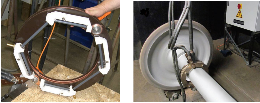
Figure 2. High current magnetization coil activated by DEUTROPULS current flow unit Left picture: Coil with integrated spraying (DB Heavy Maintenance Paderborn workshop) Right picture: Hinged coil for axle testing (Franz Kaminski Waggonbau Polska)
