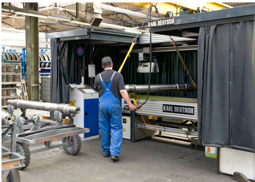
Figure 6: The cabin roof can be pneumatically opened for (un-) loading by crane The UV lamp is automatically retracted into a safety position
