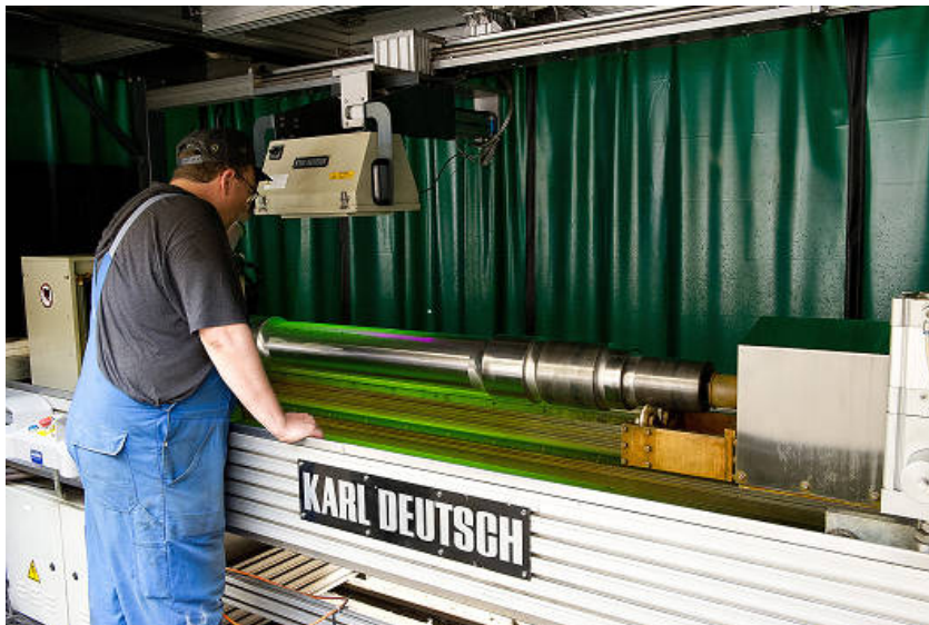
Figure 5. Motorised turning of the axle for inspection under UV light The UV lamp is smoothly fixed in a linear rail for easy movement into inspection position
