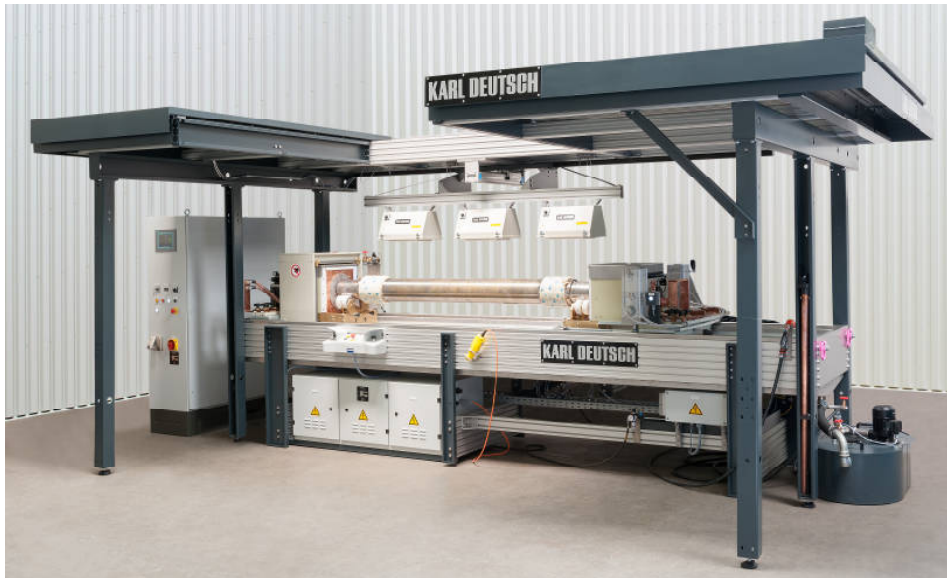
Figure 8. Special version of DEUTROFLUX UWS 3000 for testing a big variety of bogie components like wheelset, wheelset link, large spring, motor pendulum-shaft, stabilizer bar (Bombardier, D) The picture shows the cabin roof opened for (un-) loading from top by crane
