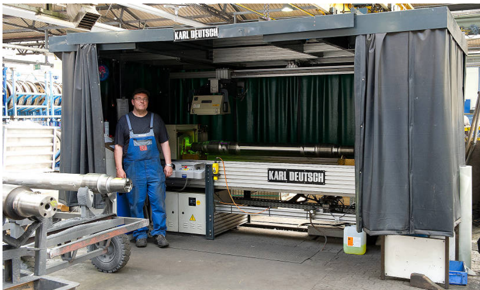
Figure 3. DEUTROFLUX UWS for railway axle test with automatic span length adjustment (DB Heavy Maintenance Krefeld workshop)
