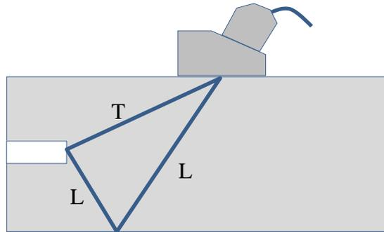
Fig. 13: Test block with vertical FBH
