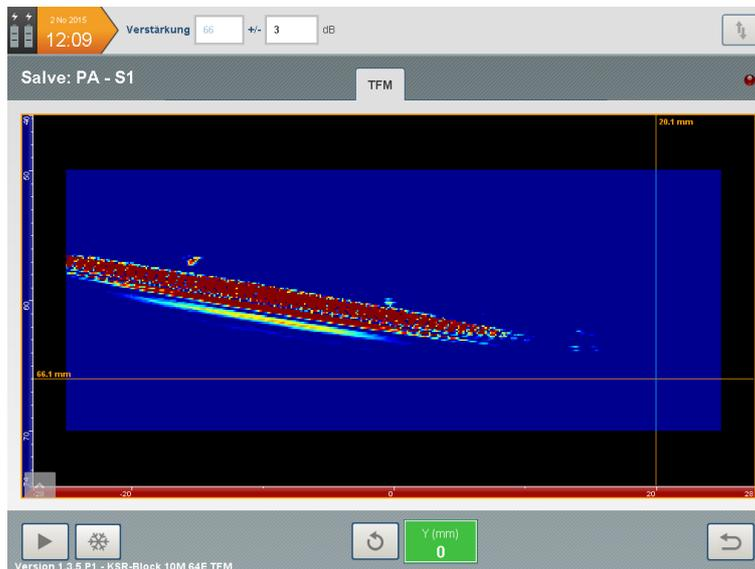
Fig. 10: Indications of the 2 FBH's at the inclined back wall
