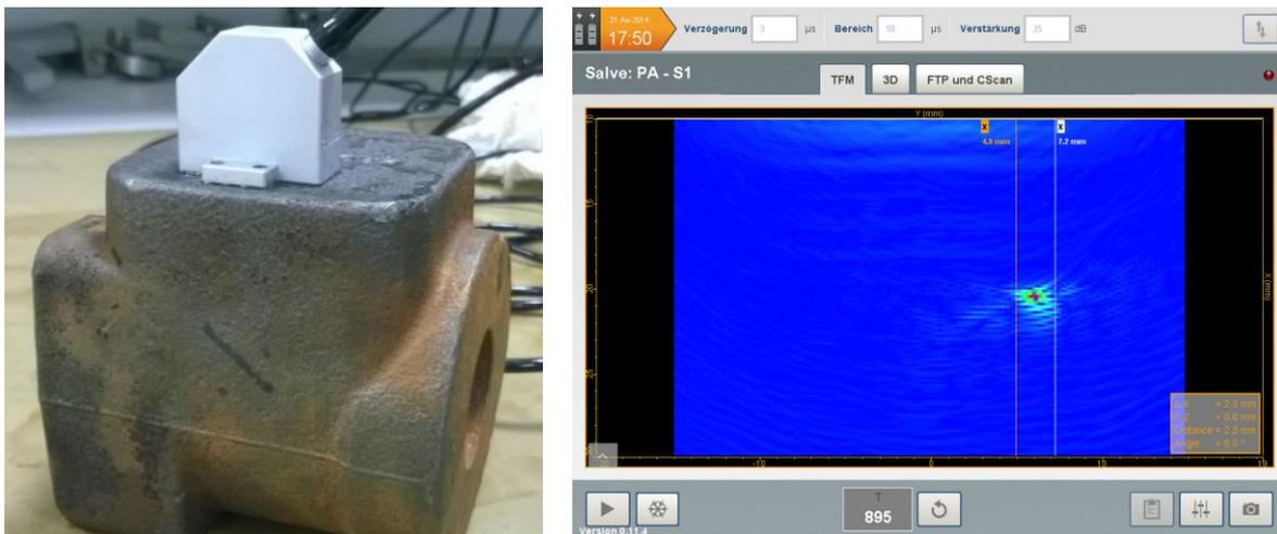
Fig. 12: Testing of castings with TFM
