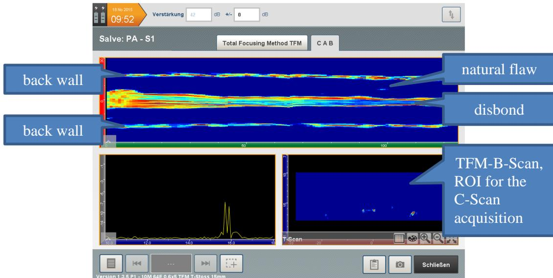
Fig. 5: C-, B- and A-Scan obtained with TFM
