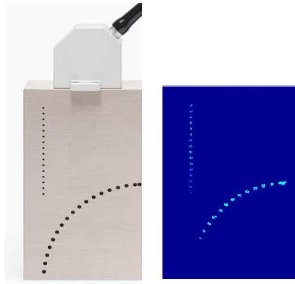
Fig. 2: ASTM block and TFM result
