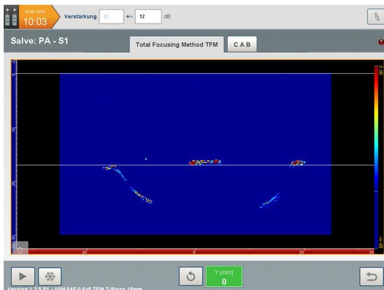
Fig. 6: Complete TFM-B-Scan: Even the weld contour is imaged
