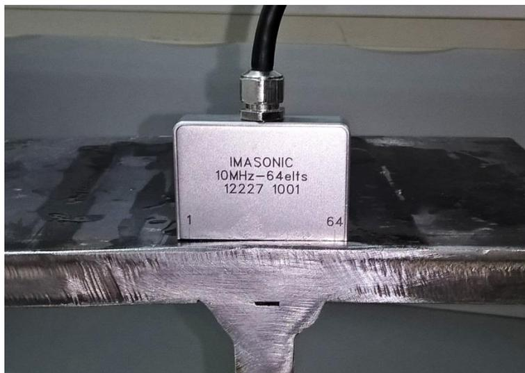
Fig. 4: Inspection of a T-joint using an array probe with 64 elements
