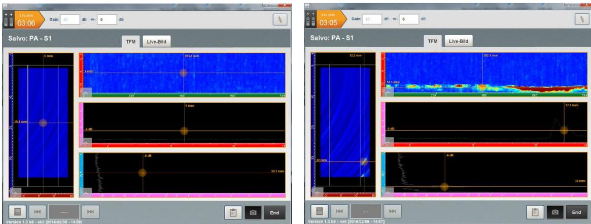
Fig. 8: TFM test results, left OK, right NOK
