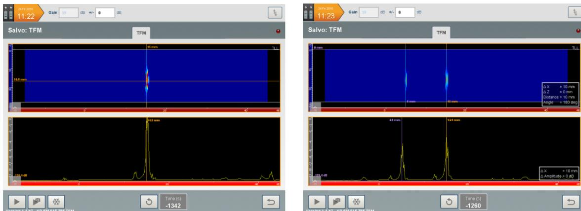
Fig. 14: Left: Indication of vertical wall, Right: Indication of vertical FBH, 10 mm in front of the vertical wall
