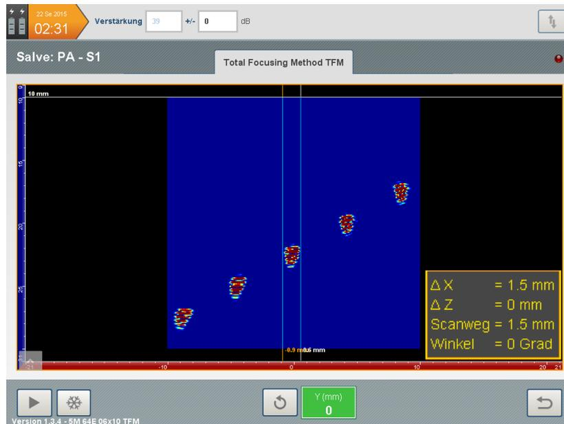
Fig. 3: Reflector size determination
