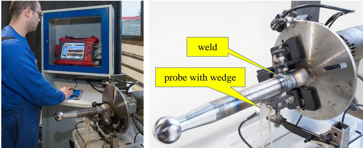
Fig. 7: Test setup for the weld inspection on tow-bars
