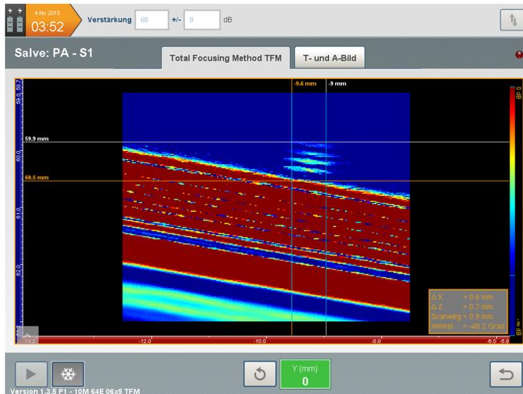
Fig. 11: Acoustically zoomed image of the FBH  $\varnothing$  0.5 mm with depth 0.5 mm
