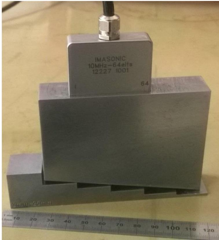
Fig. 9: Test block with inclined back wall containing 2 FBH's  $\varnothing$  1 mm (1 mm deep) and  $\varnothing$  0.5 mm (0.5 mm deep)
