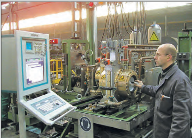
Fast system calibration using the automated sensitivity adjustment, i.e. each probe is adjusted to the same sensitivity.
