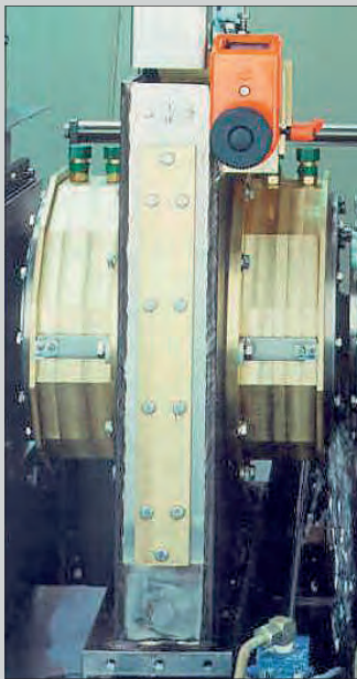
Immersion test chamber for high-speed tube testing
