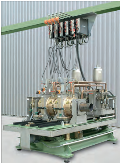
View of the test table with sliding possibility and with two immersion test chambers. The shown system is designed for tube diameters up to 170 mm. Longitudinal defects are detected and the wall thickness is measured. 40 ultrasonic channels are used.
