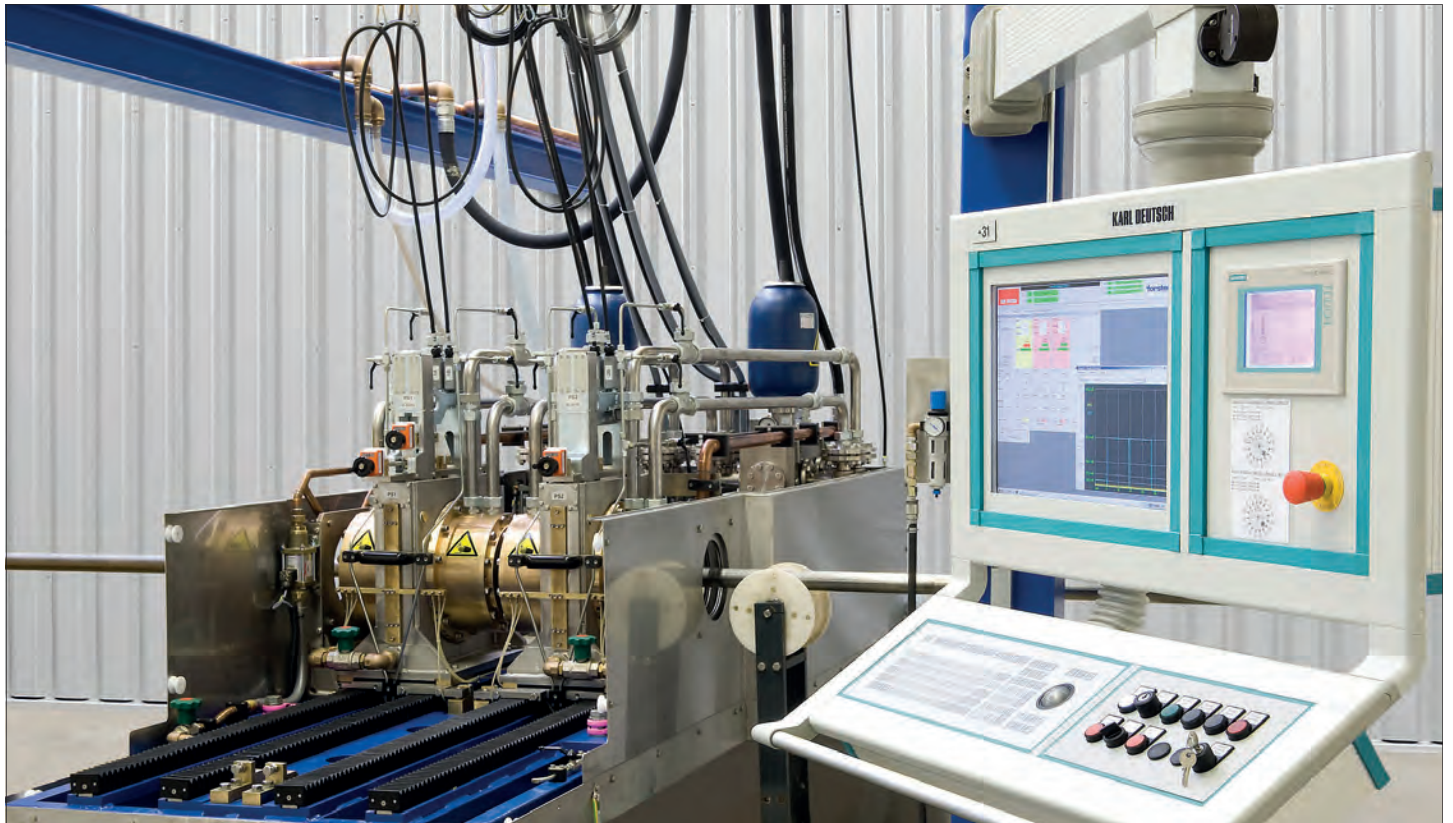
Tube testing system and operator panel to adjust the ultrasonic test parameters and the PLC parameters (Siemens).
