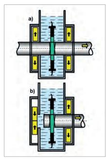
Principle of closing mechanics of test chamber: a) opened test chamber while bar is tested, b) bar is leaving the test chamber and one side of chamber is already closed. The ultrasonic probes are active as long as the bar is within the ultrasonic beams. The electronic test enable signals (to activate the probes) are programmable to reach the shortest possible untested ends.
