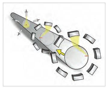
Since invention of the HRPS-setup, many probe configurations have been realized. For bar testing, a setup with 16 angle beam probes and 5 straight beam probes has been proven to be a reliable setup for 100% cross sectional coverage of the bars. The more probes are used, the higher is the probability of detection (POD) also of oblique and crack-type defects.
