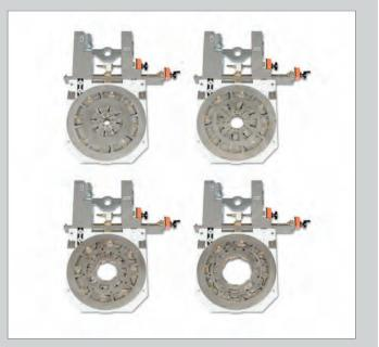
Test cassette with ring of ultrasonic probes: Angle beam probes are used to detect surface defects while straight beam probes are used to detect core defects. The testing angle of all angle beam probes is centrally adjusted by the spindle and the orange dial.
