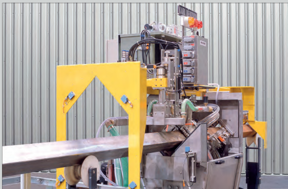
ECHOGRAPH-KNPS billet testing system: Light barriers check the billet position.
