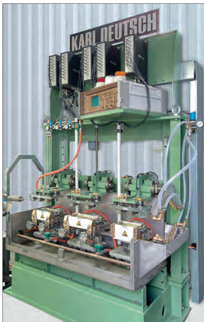
View of inspection system with three test chambers (longitudinal and transverse defects, wall thickness).
