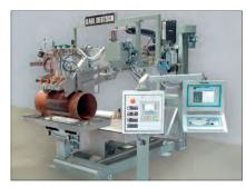
Online Testing System for ERW-Pipes: The probe holders can be moved between the testing position and the calibration position. In the calibration position, a short pipe segment is used for the sensitivity setting of all probes.
