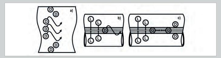
Typical testing tasks for the ERW-pipe inspection.
