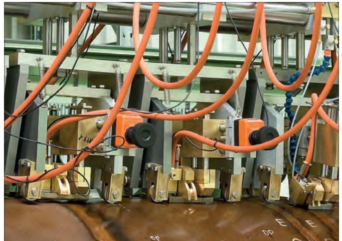
Probe holders for the detection of laminations in the heat-affected zone
