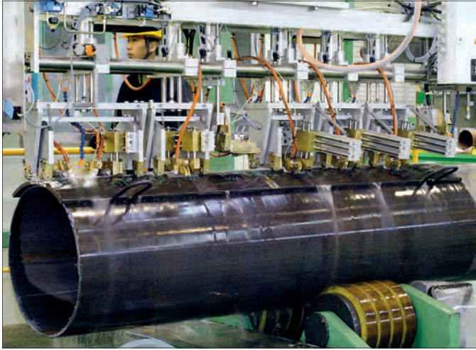
Probe holders of weld test system on pipe segment for system calibration (photo courtesy of EEW-Korea)
