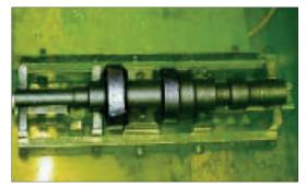
Testing of forged gear shafts (chevrons)
