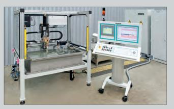
ECHOGRAPH test electronics with immersion tank, probe manipulator and water filter circulation system: The operator panel contains a touch screen for setting the PLC parameters and an industrial keyboard to set the ultrasonics.
