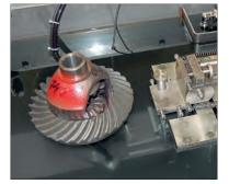
Testing laser-welded gears
