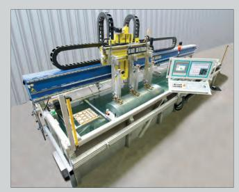
Test tank for rotational aluminium billet inspection
