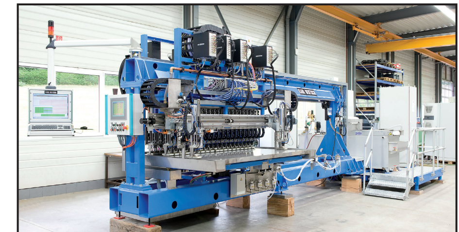
BAPS strip testing system, 100%-coverage
