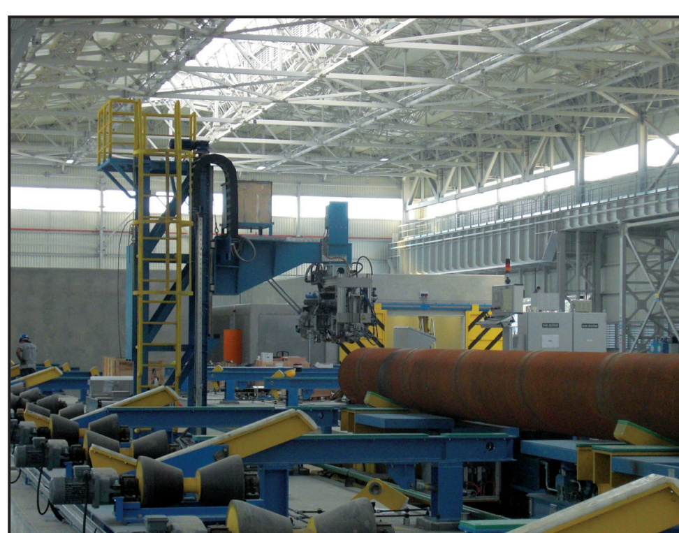
SNUS weld testing system with machine stand and pipe
