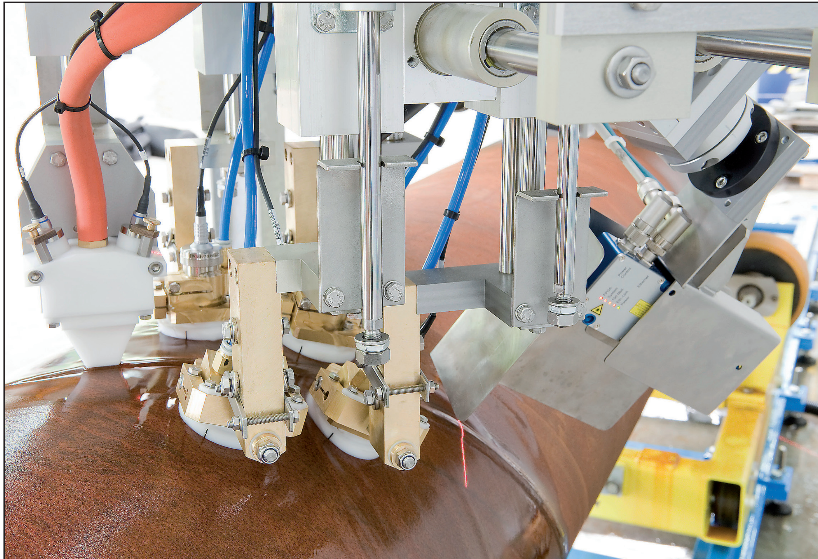
SNUS first weld testing system: 6 probes (4 longitudinal, 2 transverse), laser-based seam tracking
