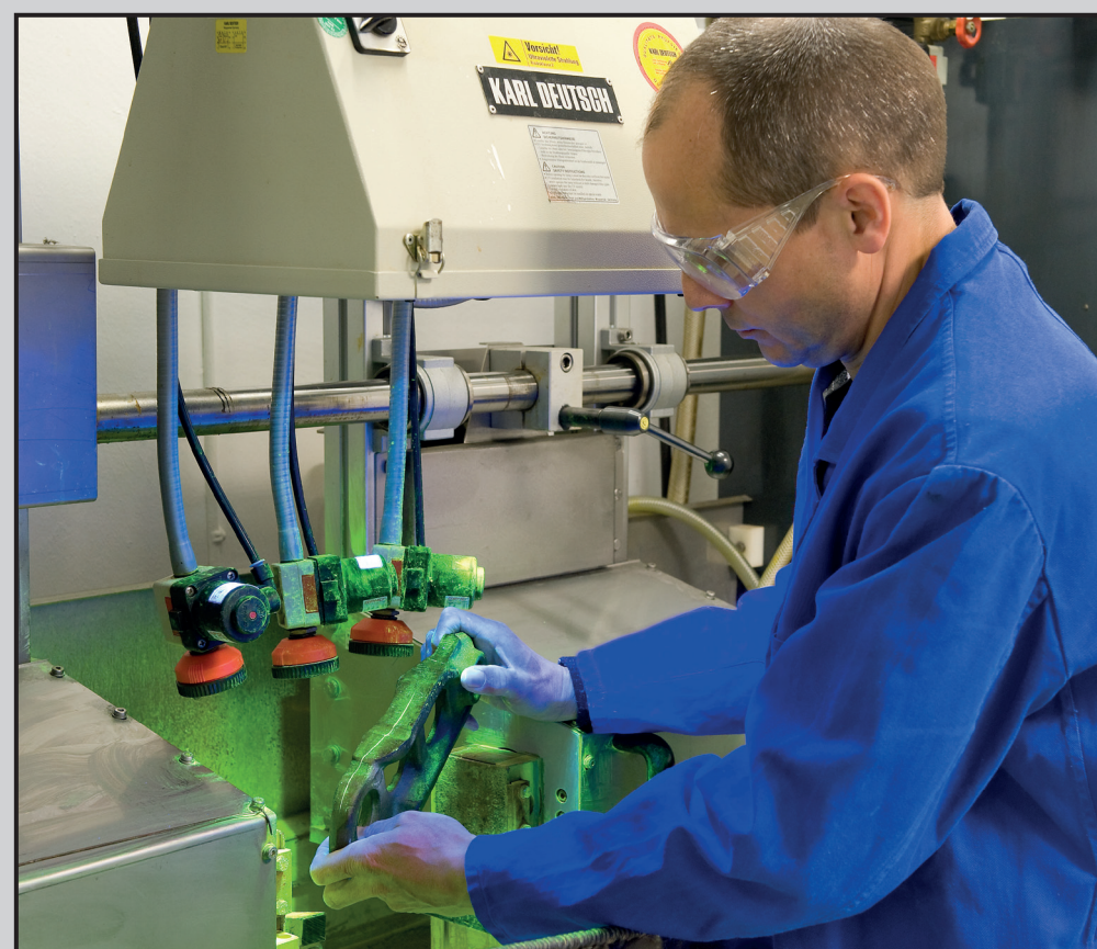
Crack evaluation under UV light
