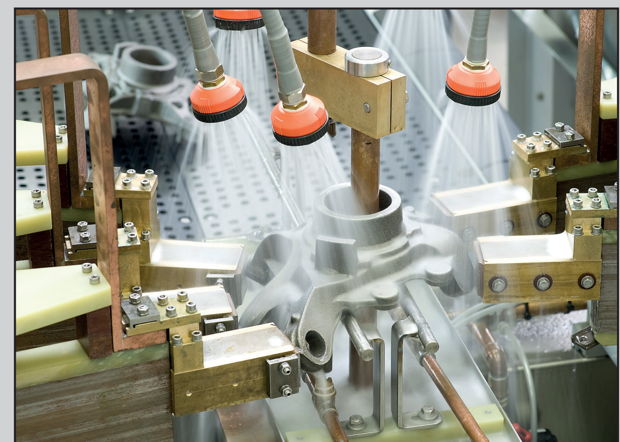
Testing of steering knuckle (6 contacts, ejector)
