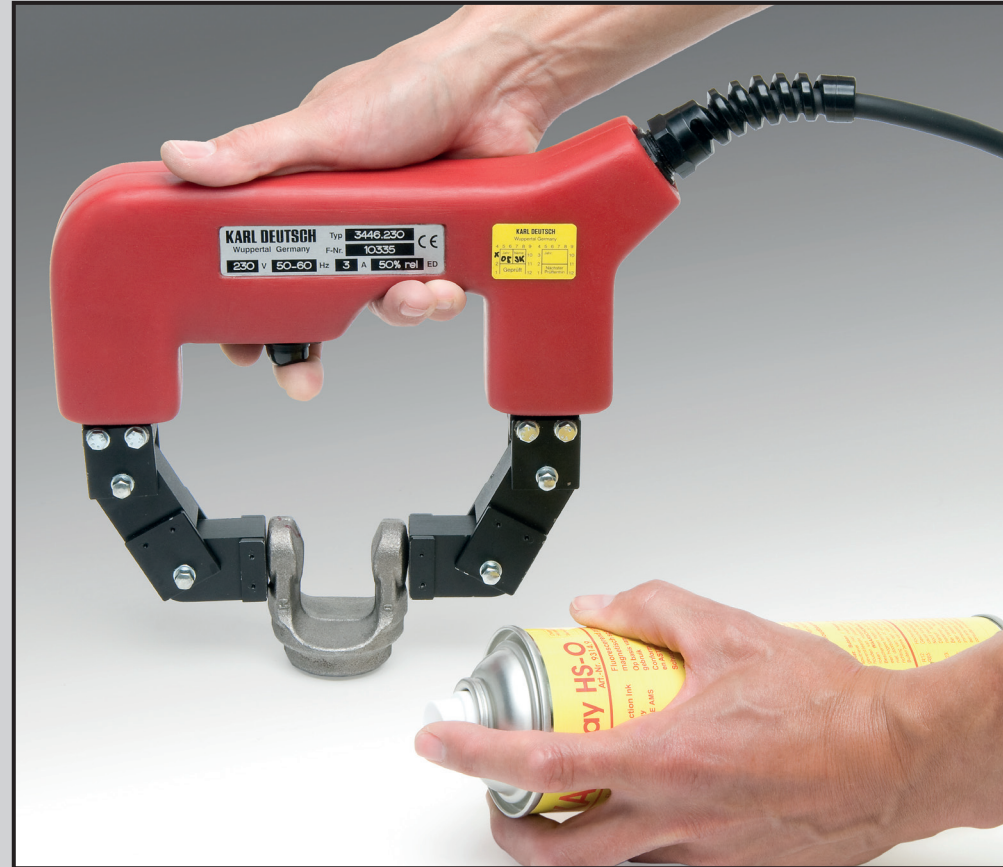
Testing of forged parts with flexible attachment poles
