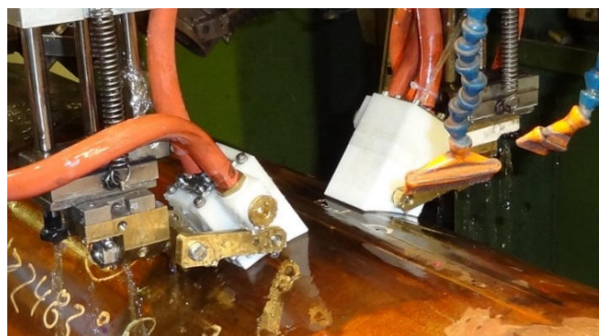
Fig. 2: Squirter probes for the detection of longitudinal flaws
