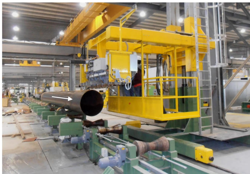
Fig. 8: Test system with moving pipe
