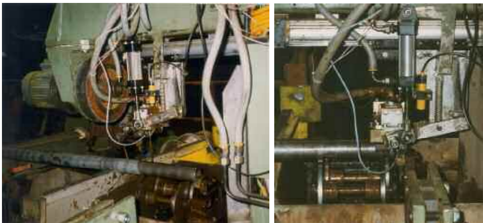
Figure 12: Pipe-end inspection, a) lifted probe holder above tube, b) lowered probe holder during test of rotating tube.
