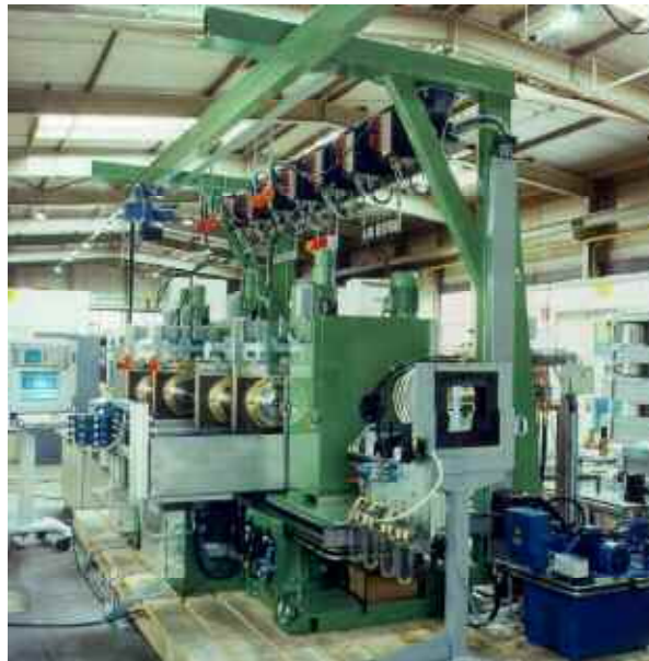
Figure 1: Full-body tube inspection with the HRP-System with a testing speed of up to 2 m/sec.
