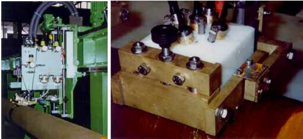
Figure 11: Test traverse for tube testing, a) traverse with multi-probe holder for lamination testing, b) multi-probe holder for the simultaneous testing for all flaw types (longitudinal, transverse & laminations).
