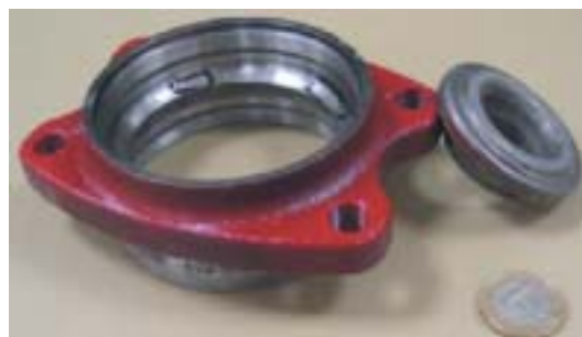
Figure Bearing Testing , the edges within the bearing surface make an ultrasonic test impossible.
