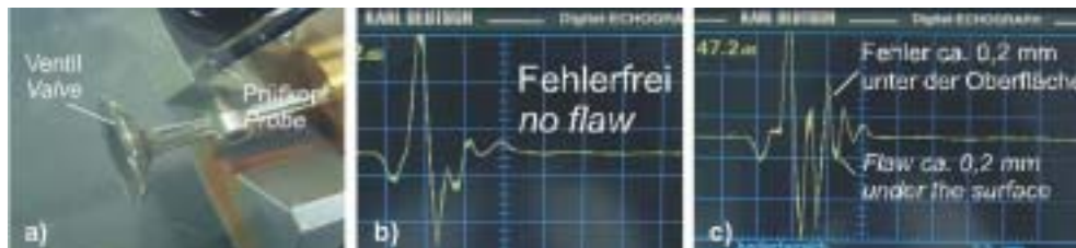
Figure Valve Testing , a) immersion test setup, b) a-scan without defect, c) echo from small near-surface defect.
