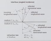
Ultrasonic testing is applicable for the detection of internal flaws like inclusions and cracks, often for weld testing. But it is also applicable for the measurement of
