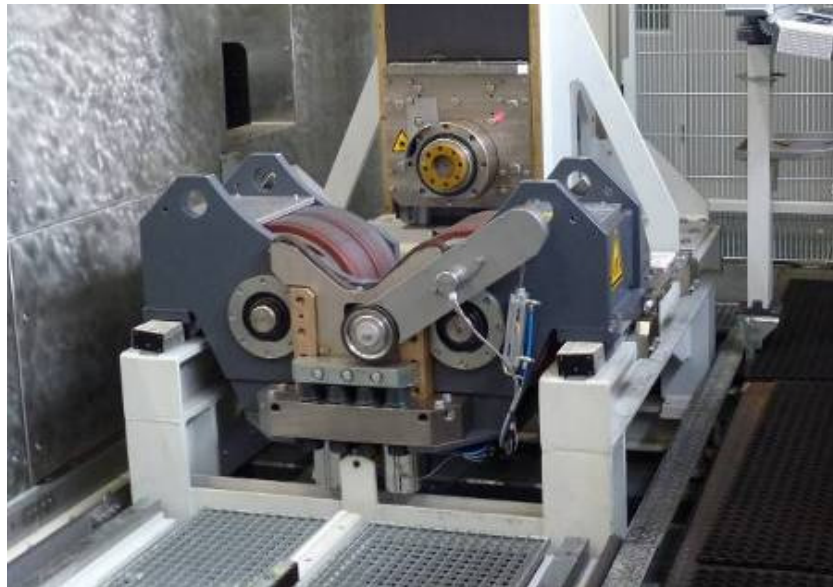
Figure 7. Roller devices with damping modules for large component weights
