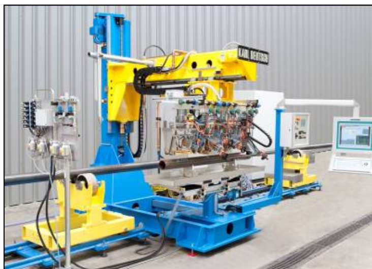
Figure 10. Conventional online weld testing system (this example with 8 probes). The probes are moved offline above a short tube sample for calibration.
