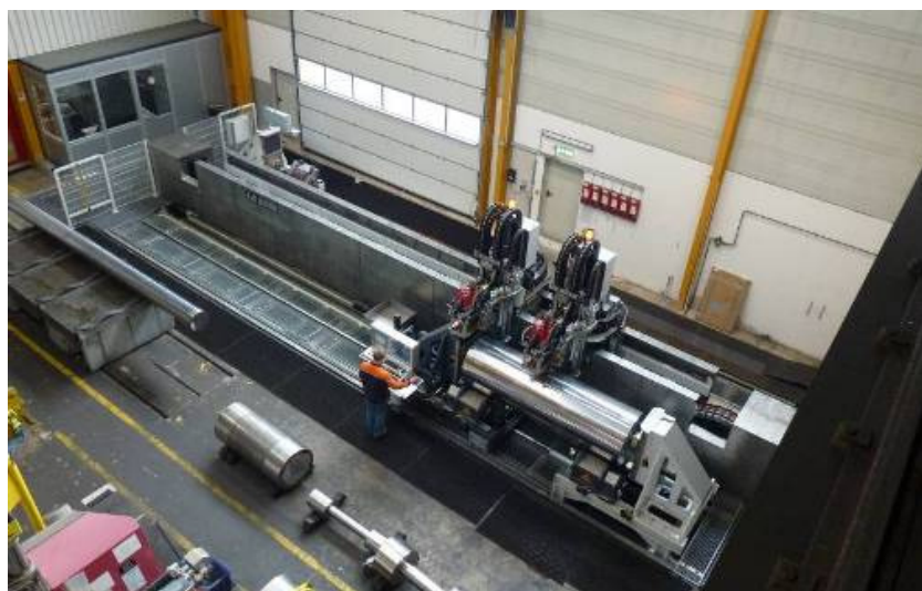
Figure 6. View of the newly developed ultrasonic testing system in the turning shop No III of BGH Edelstahl Siegen GmbH
