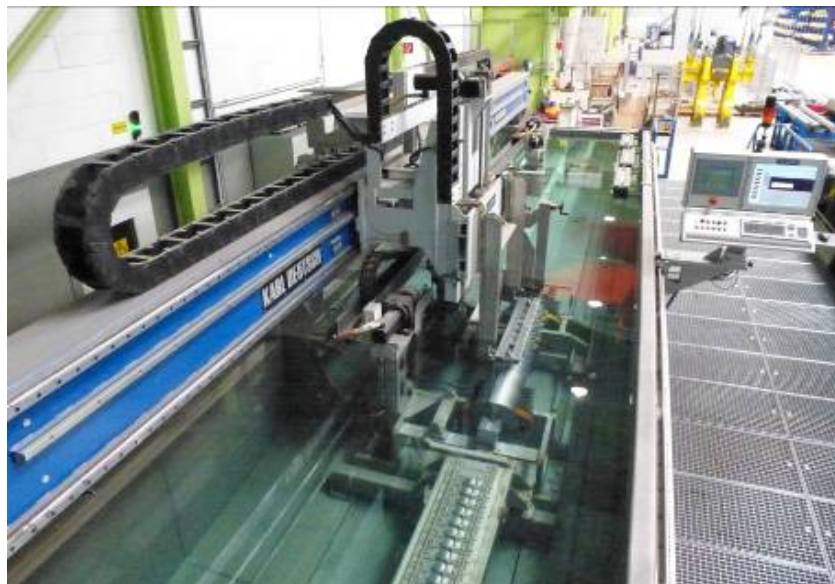
Figure 3. View of immersion tank testing system for aerospace bars (titanium or nickel alloys)
