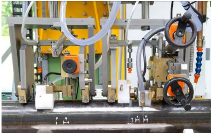
Figure 12. Three phased array probe holders with white plastic water nozzles
