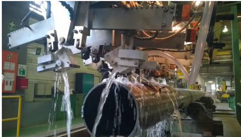
Figure 13. Probe holders for LSAW-pipe weld testing system. Two phased array probe holders are provided for longitudinal defect detection.
