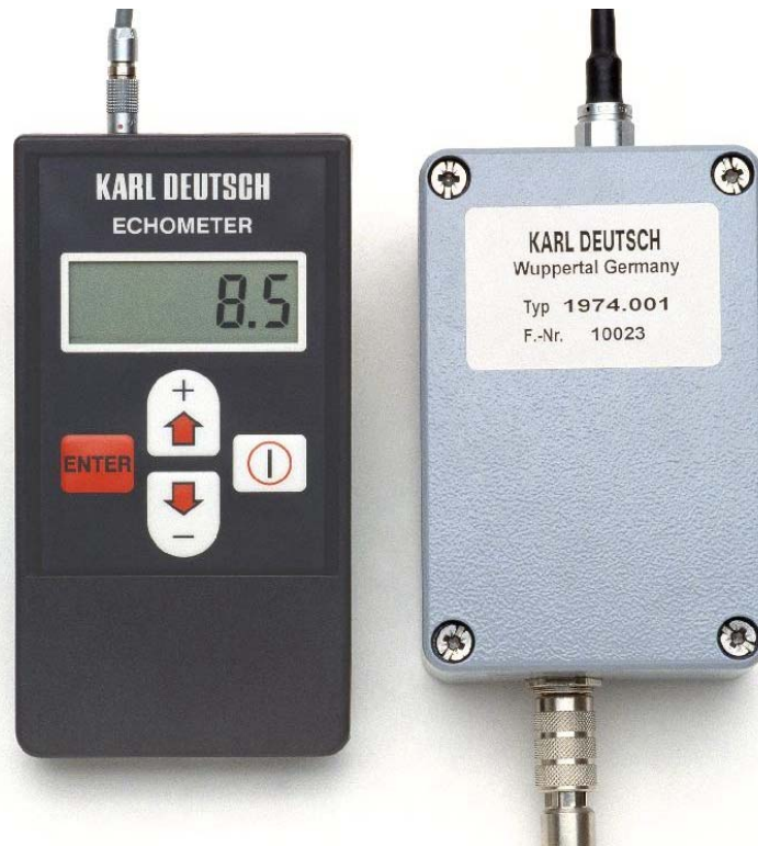
Fig. 1: ECHOMETER-host station with data display (left) and on-site wall thickness electronics (right).
