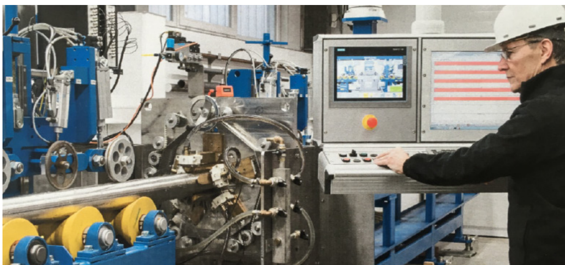
Fig. 11: ECHOGRAPH STPS PAUT system with five PAUT probes and water jet coupling
