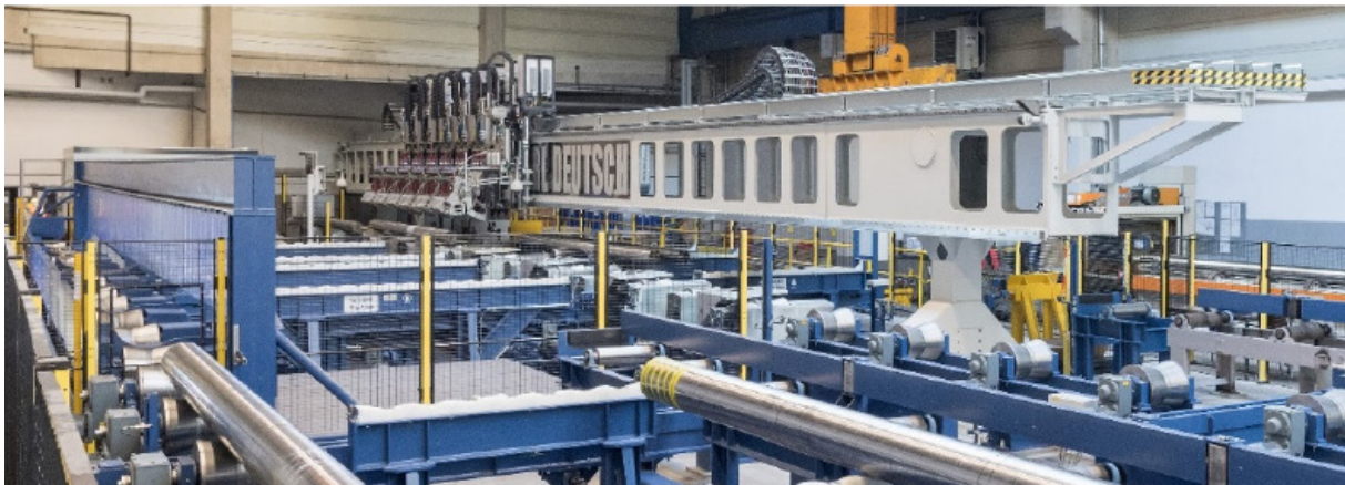
Fig. 12: Testing Bridge for steel bars at BGH-Siegen Edelstahl GmbH. The bars are loaded from the right side crosswise below the white bridge via lifting bars. The roller conveyor for sorting purposes and the station for reworks are shown left in the figure.
