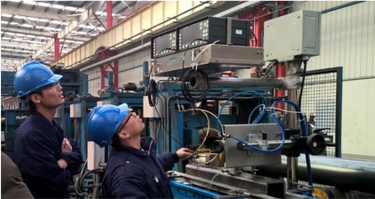
Fig. 3: A two-channel rf-weld inspection for the process control on endless tube (below right in the picture)
