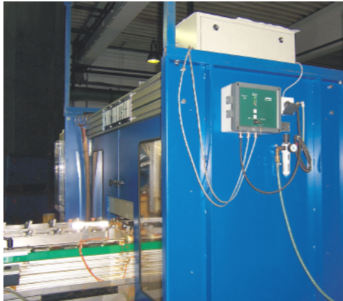
Fig. 7: Onsite Installation of FLUXA-Control in a well-known foundry, carried out as a retrofit to the existing DEUTROMAT testing system.
