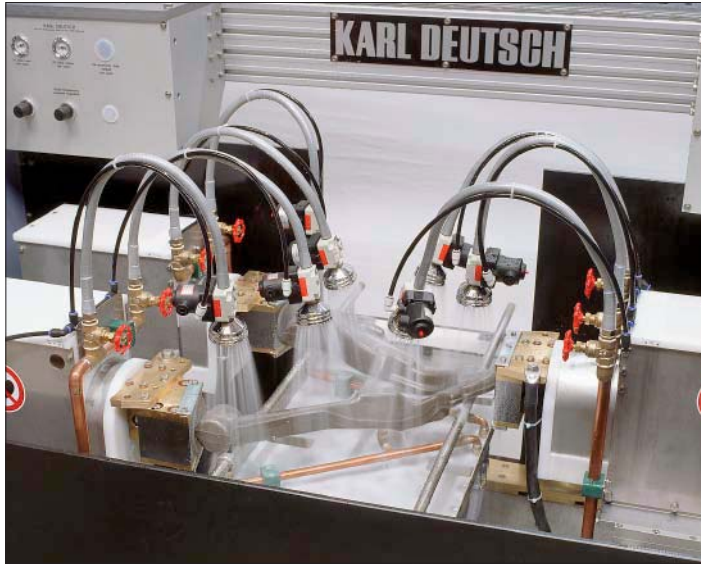
Magnetization of a transverse control arm with three contacts
