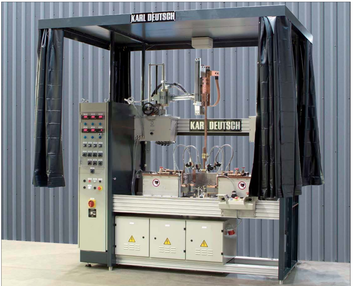
General view of a DEUTROMAT Multi-Contact machine. A close-up of the test part is shown on the front page of this leaflet. Visual inspection of the test parts can be done directly in the machine. If necessary, a darkening cabin can be mounted.
