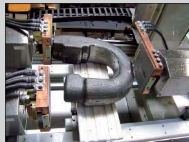
Test machine with moving coil and three current contacts for magnetization of large hooks
