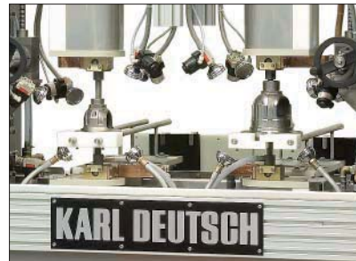
Magnetization of two housings with two vertical magnetization stations
