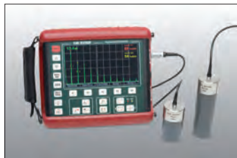
Adjusting standards with echo sequences of 50 mm and 100 mm
