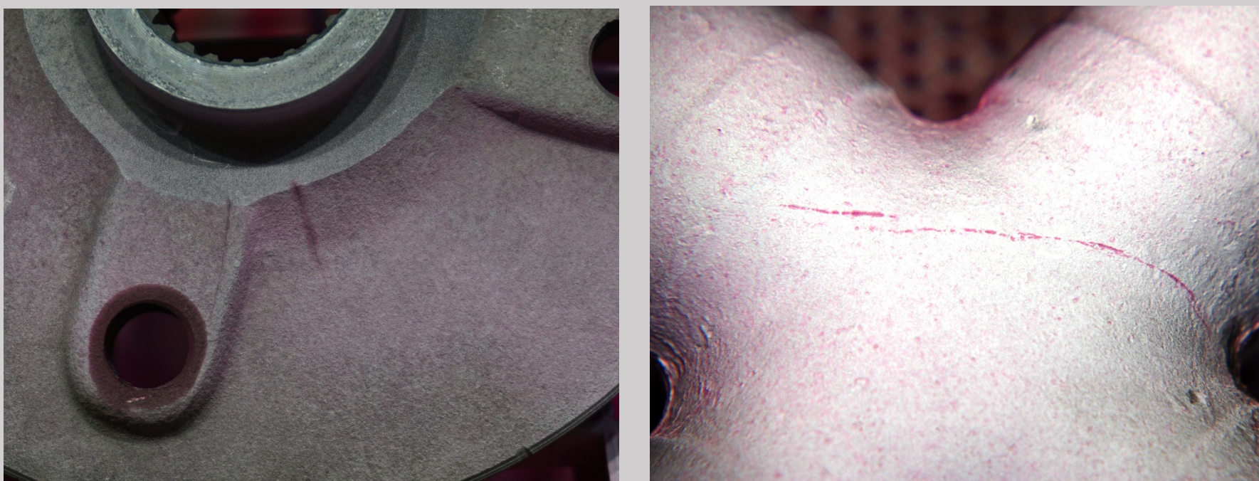
Test results with the dye penetrant testing (red/white). The developer application on a forging is insufficient. The contrast between background and display is considerably reduced (left). The uniformly covering developer layer on the casting provides a good color contrast (right).
