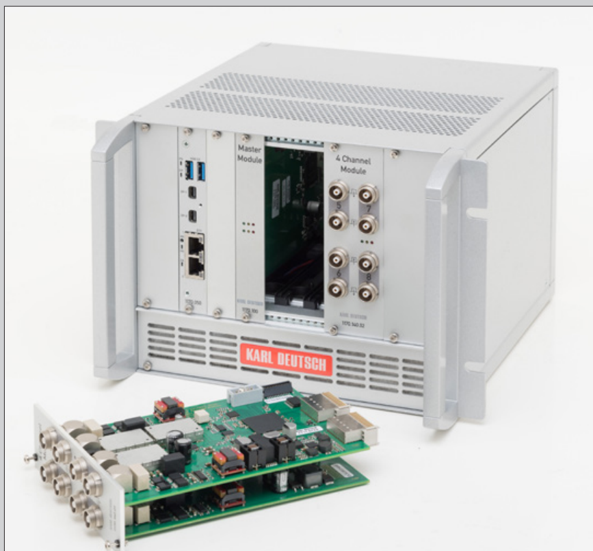
The ECHOGRAPH 1170 testing electronics is based on very compact, four-channel modules that are interconnected according to the number of channels. Since special through-transmission methods are also supported (e.g. for nodularity testing on castings), eight LEMO sockets can be seen.
