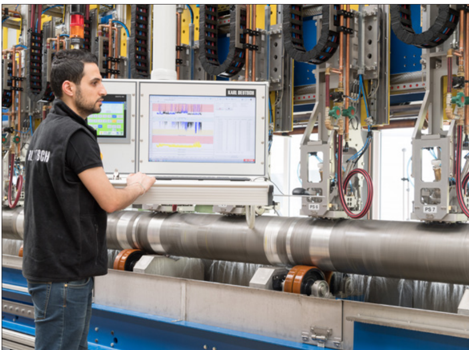
Convenient adjustment of the testing system by a laterally movable control panel
