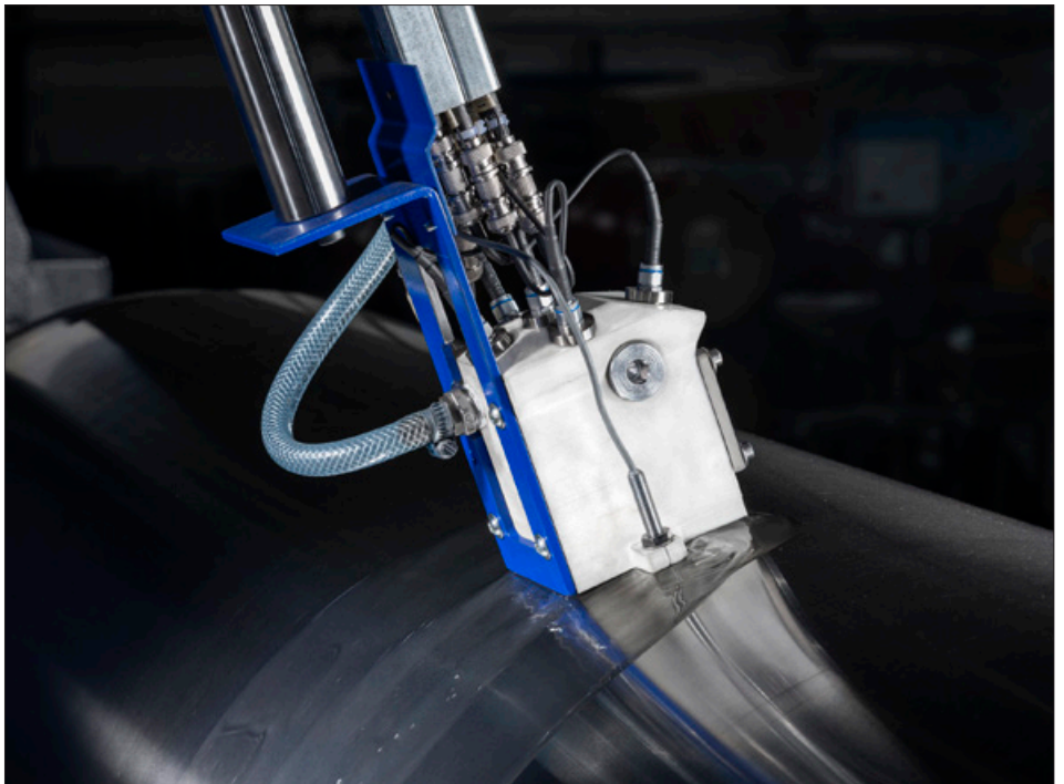
Probe holder with flow water coupling, equipped with five ECHOGRAPH ultrasonic sensors for roller inspection
