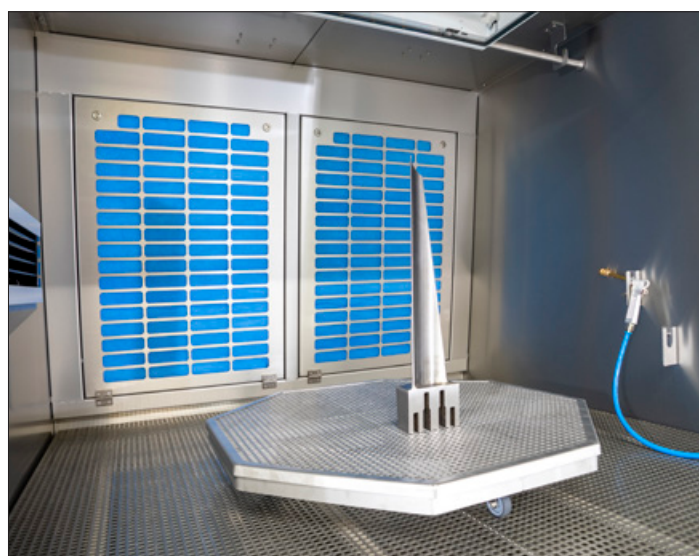
Test chamber with turntable and internal connections for water and compressed air (with a laboratory test part)
