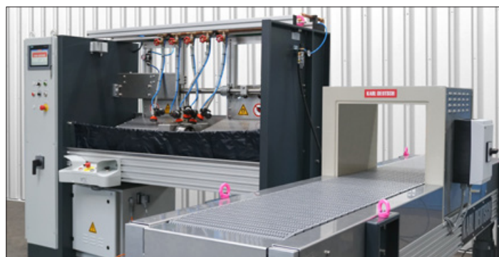
Conveyor belt with integrated ESV demagnetising coil
