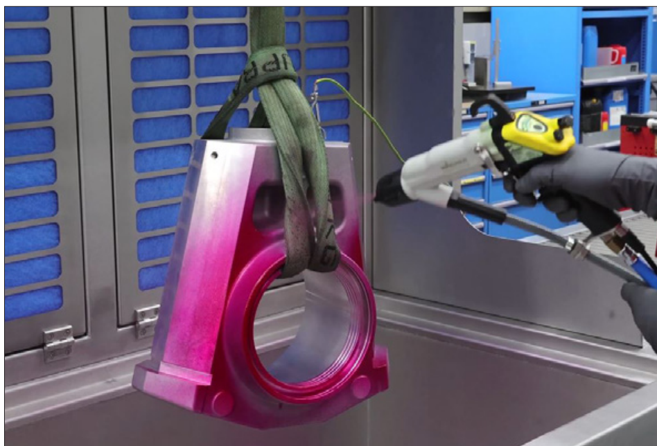
Electrostatic application of test agent at the penetrant station
