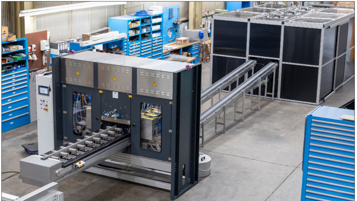
DEUTROMAT chain conveyor – general view (from left to right: infeed area, magnetisation station, conveyor belts, darkening cabin)
