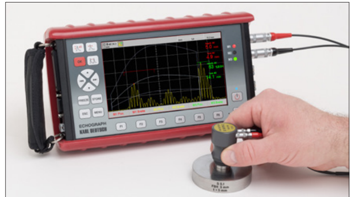
DGS-test via TR-probe with active backwall echo drop
