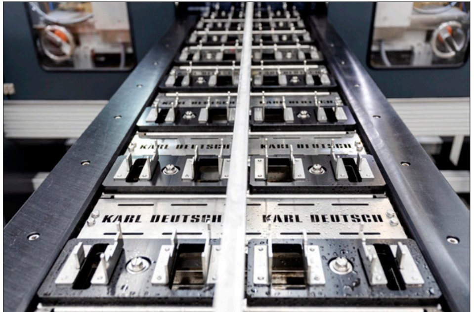
Individual, quickly convertible workpiece fixtures at the infeed of the MT system
