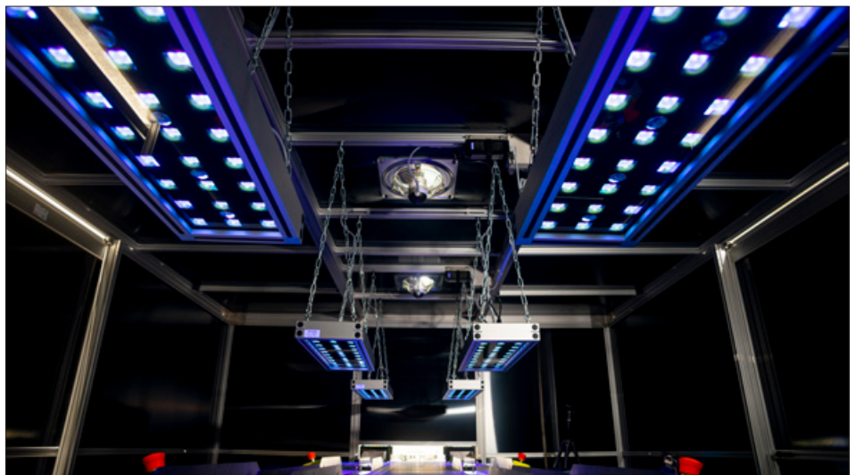
Darkening cabin with six operator positions, each equipped with a large-area UV-LED lamp
