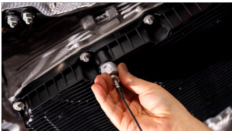
The ultrasonic sensor is connected to the gearbox oil pan via a bayonet mount.
