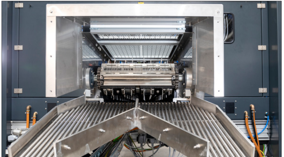
Outlet side of the magnetisation station with spatial separation and transfer of the magnetised and rinsed parts to the conveyor belts
