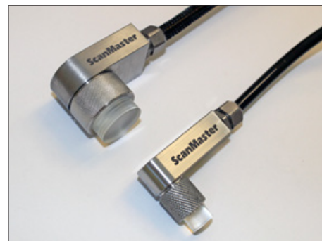
Comparison of both available probes: on the left for a diameter up to 16 mm, on the right for a diameter up to 9 mm
