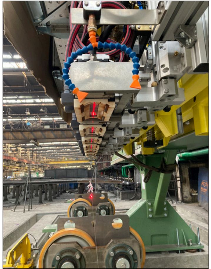
Laser technique and justify lines are used to check the alignment of the test bridge to the turntable stations.
