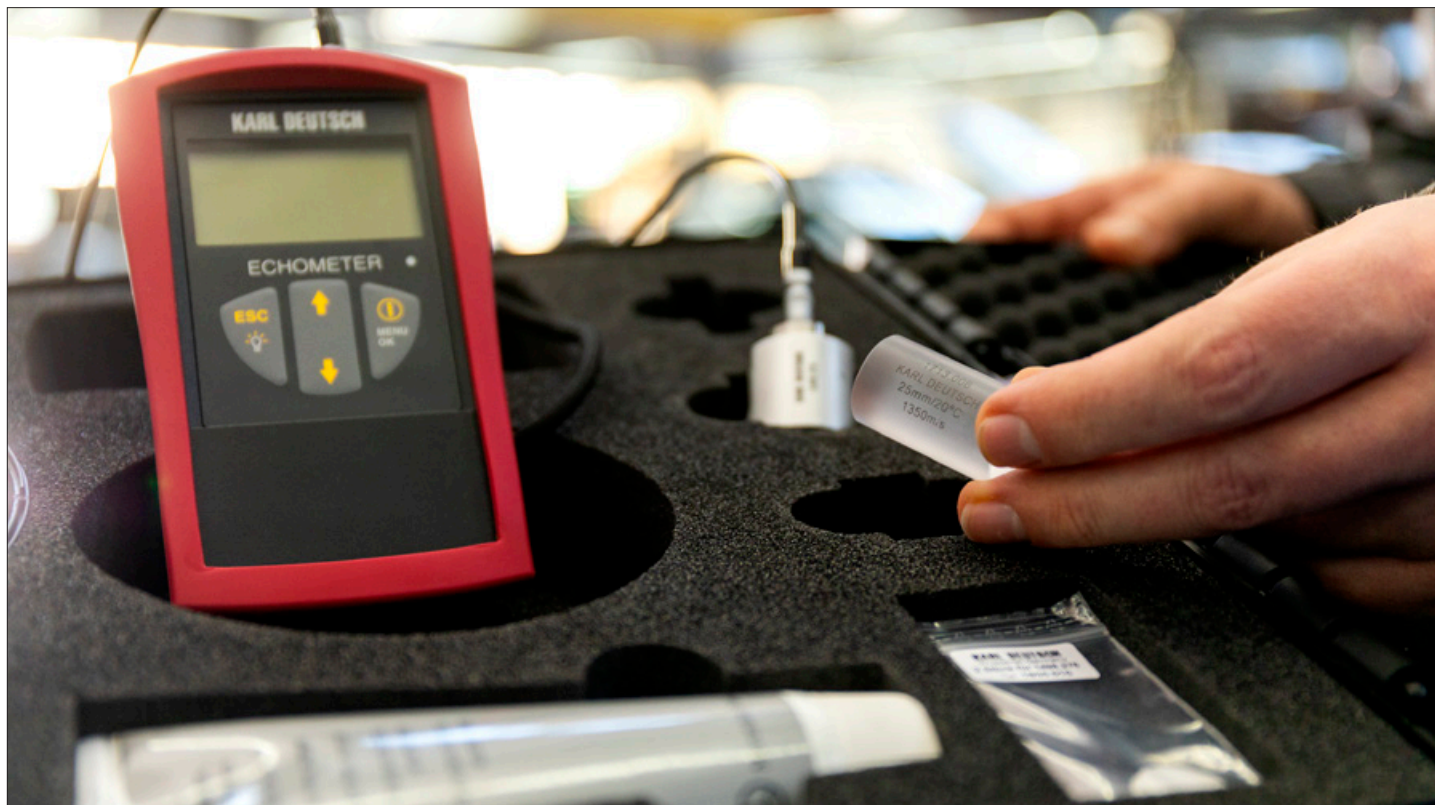
New development for Mercedes-Benz: An innovative ultrasonic measuring instrument for measuring the transmission oil level
