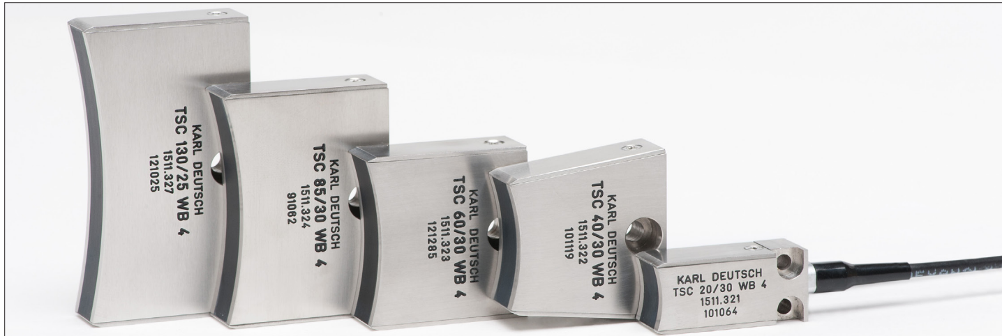
Special line-focussed probes for angular incidence in different sizes to test the respective tube diameters. Each probe covers 18 – 30 degrees of the tube circumference. In dependence to the tube diameter 16 to 20 probes are provided for full ultrasonic coverage.
