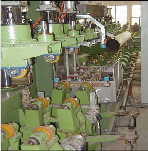
Examples for the helical tube conveyor which must provide a transport of the tubes without vibration. The rotational and the linear tube speed must be perfectly synchronised for the respective tube diameter. Therefore, the angles of the supporting rollers (below the tube) and the pressure rollers (above the tube) are adjustable with respect to the tube axis.
