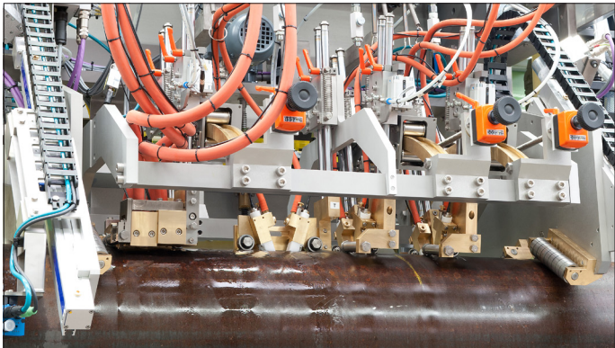
In this example ten probes are used for offline weld testing. The six angle beam probes use water jet coupling (also called squirter technique). The incidence angle can be adjusted without steps for a perfect setting with respect to pipe diameter and wall thickness and without changing the probe.
