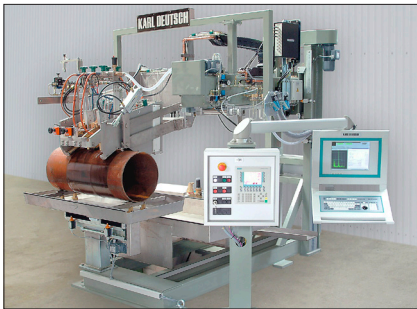
Online Testing System for ERW-Pipes. The probe holders can be moved between the testing position and the calibration position. In the calibration position, a short pipe segment is used for the sensitivity setting of all probes.
