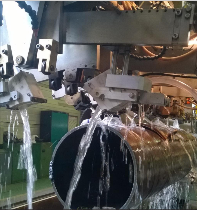
Upon customer request one (or all) test functions can also be implemented using the phased array technique (picture courtesy of EEW-Germany).
