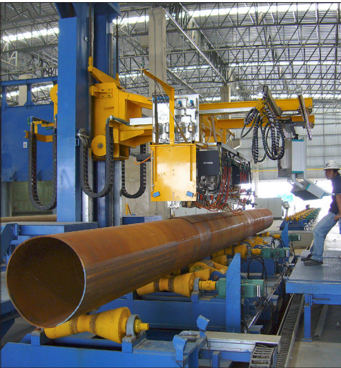
The testing mechanics with the probe holders is mounted to a stable machine stand. The ultrasonic probes are positioned near the weld seam in the 12 o'clock position and symmetrically to the weld seam. The height of the horizontal boom (in yellow) and the ultrasonic probes are pre-positioned in accordance with the pipe diameter.
