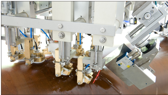
The weld seam is continuously monitored by a laser-optical tracking system.
