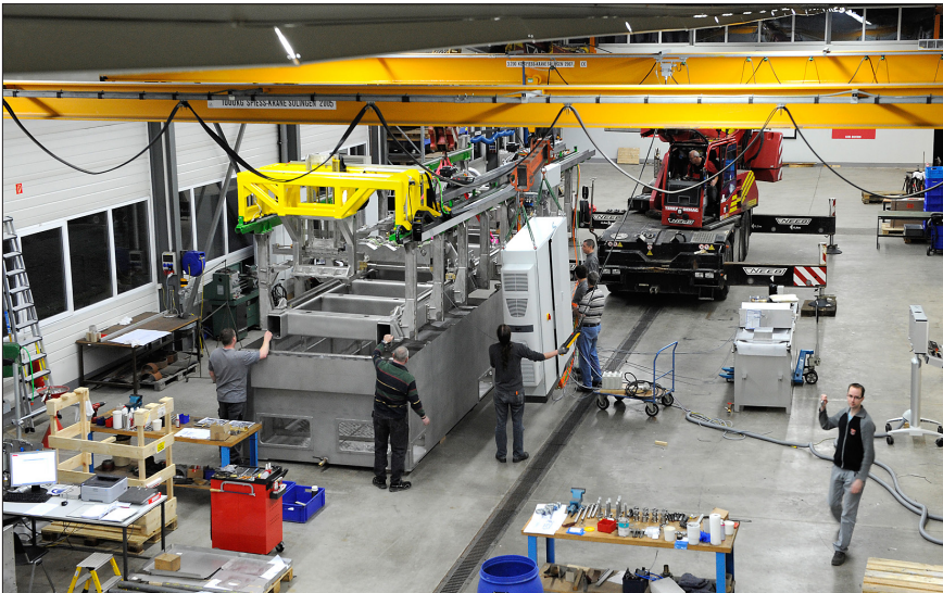
View into the systems workshop where a large immersion test tank is assembled
