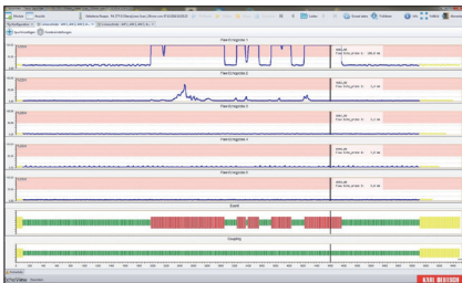
ECHOVIEW GUI with strip charts and assigned event and coupling information
