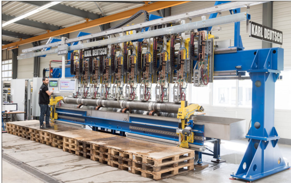
Testing portal for round casted aluminium billets with ten straight beam probes for core-defect detection in accordance with ASTM B 594-90. In addition, angle beam probes inspect the billets for surface defects.
