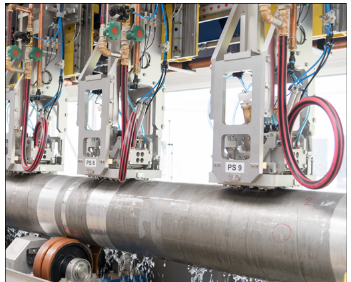
Here, each probe holders contains one straight-beam probe. The surface of this aluminium billet is as casted and therefore quite rough. A large metal skid protects the probe and the water nozzle from damage.
