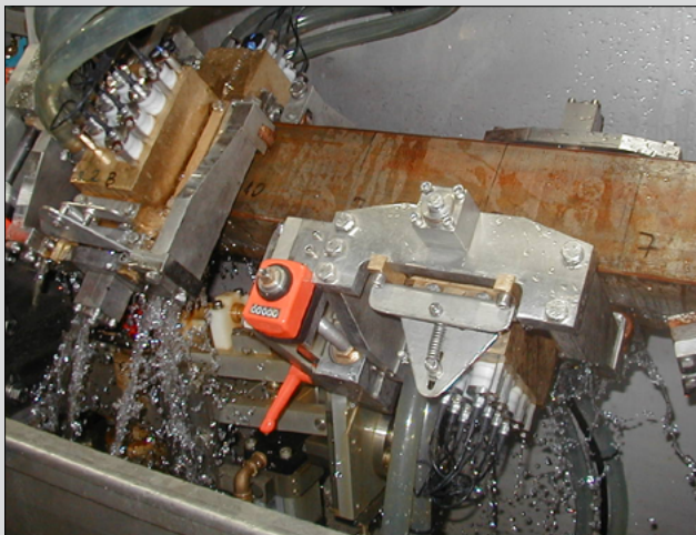
Four probe holders for quadratic billets, each carrier with seven probes and positioning from all four sides. The guidance is achieved by guiding rollers and hard-metal skids.
