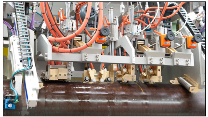
Example application: Ten probes for offline weld testing, six angle beam probes with water jet coupling. The incidence angle can be adjusted steplessly for perfect settings without changing the probe.
