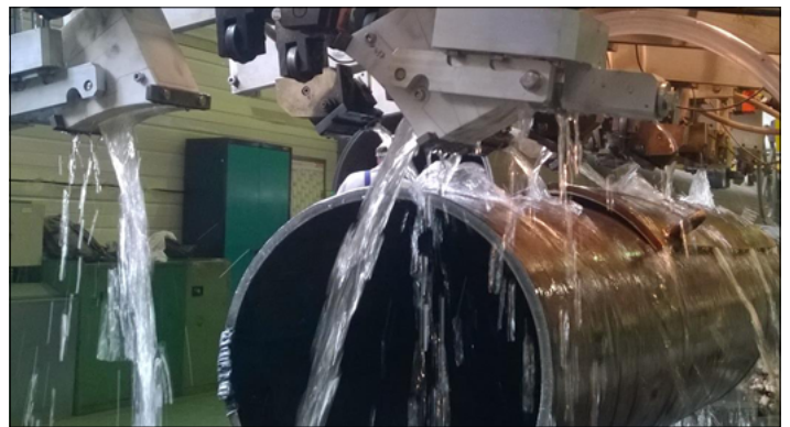
Upon customer request one (or all) test functions can also be implemented using the phased array (PAUT) technique (picture courtesy of EEW-Germany).
