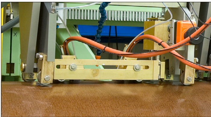
Probe holders for the on-bead detection of transverse defects: Water jet coupling enables the positioning of the probes directly on the weld crown.
