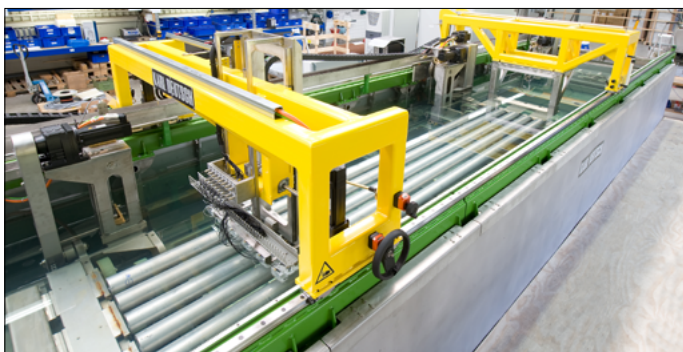
Large immersion test tank for bars, profiles and tubes. Up to six samples can be tested at the same time.
