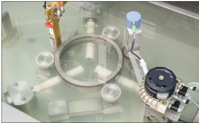
View into immersion tank with bearing ring. The probe holder is positioned outside the ring to inspect the internal ring surface. For higher throughput, four similar probes are used for the inspection. The ring is put into rotation with three rollers. A vertical probe movement results in helical test tracks.
