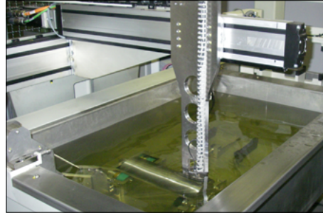
Steel cleanliness test (SEP 1927)
