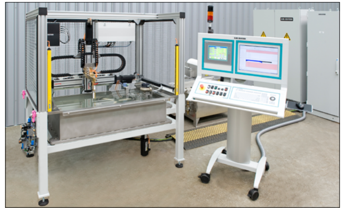
Immersion test tank with probe manipulator, water filter circulation system and ECHOGRAPH testing electronics. The operator panel contains a touch screen for setting the PLC parameters and an industrial keyboard to set the ultrasonics.
