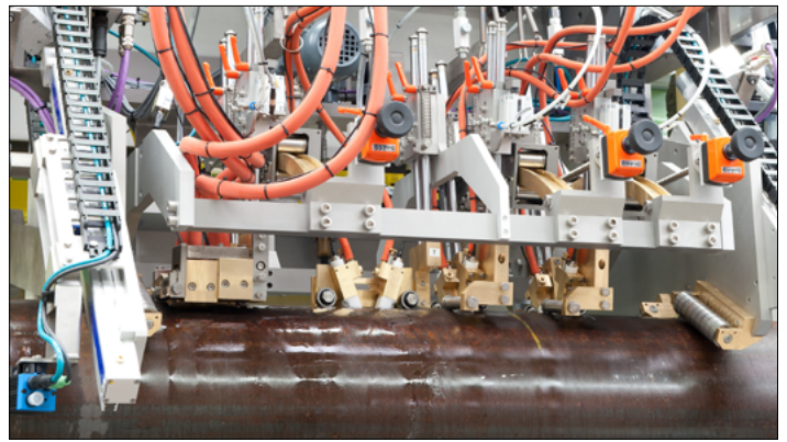
Example application: Ten probes for offline weld testing, six angle beam probes with water jet coupling. The incidence angle can be adjusted steplessly for perfect settings without changing the probe.
