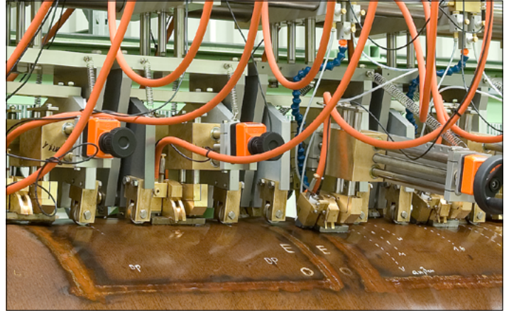
Probe holders for the detection of longitudinal defects: Spindles with position gauges are used to adjust the distance between the probes and the weld seam.
