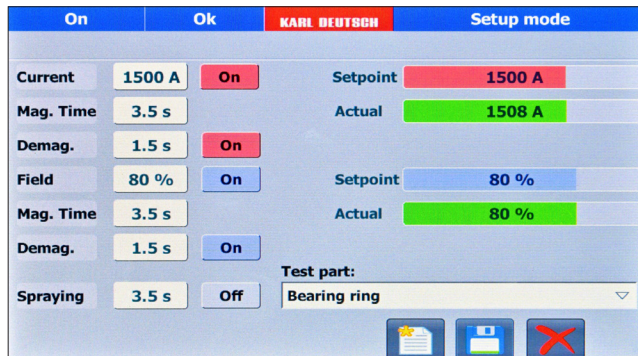
MEMORY: 7" touch panel for setting all parameters
