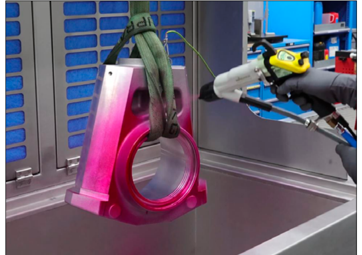
Testing agent application with electrostatics at a penetrant testing station
