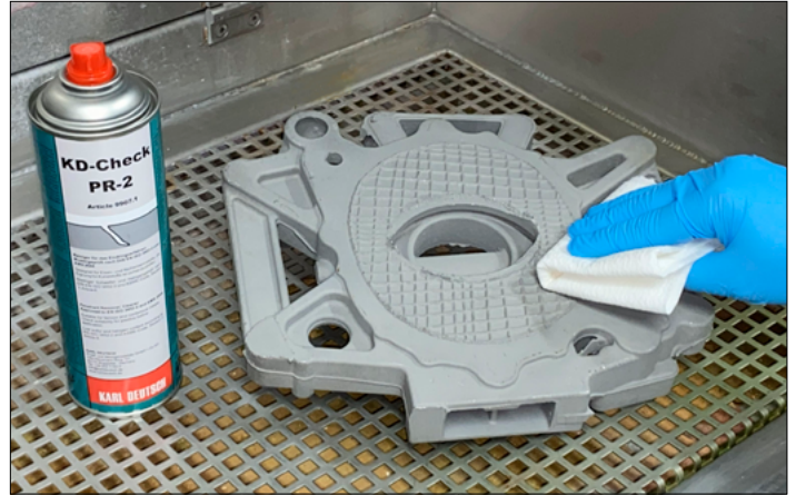
Pre-cleaning of a test piece with KD-CHECK PR-2
